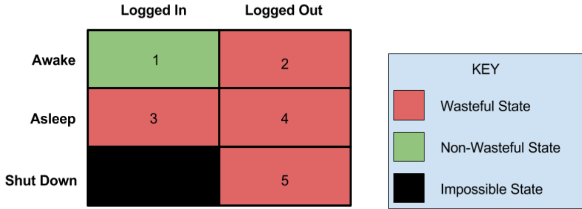
Figure 18: A visual representation of the five desktop computer states and their respective categorization as wasteful or non-wasteful.
