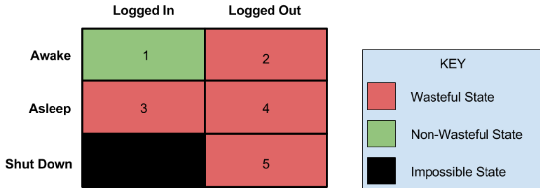
Figure 1. This figure illustrates the five desktop computer energy states and classifies each as either wasteful or non-wasteful.
