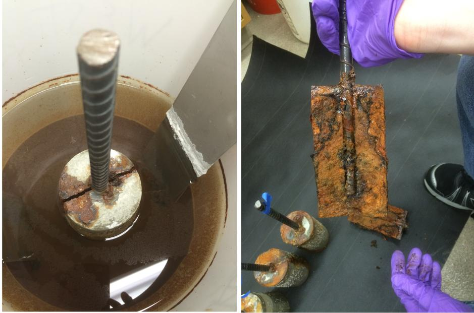
Figure 21: One of the corroded samples for unmodified epoxy coating
