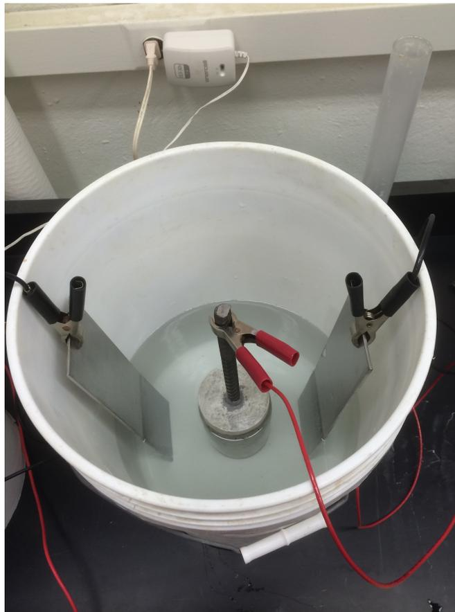
Figure 5: Setup for accelerated corrosion testing
