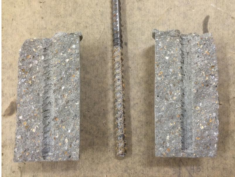
Figure 18: A broken sample by pullout testing coated with self-healing coating with 20 wt.% microcapsules
