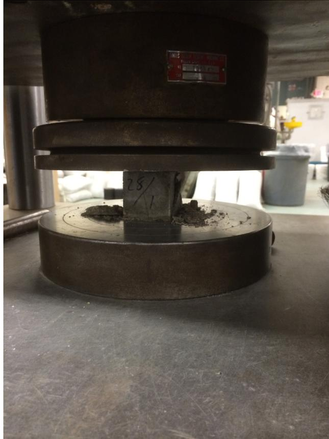
Figure 4: Compression testing for a 28-day concrete cube
