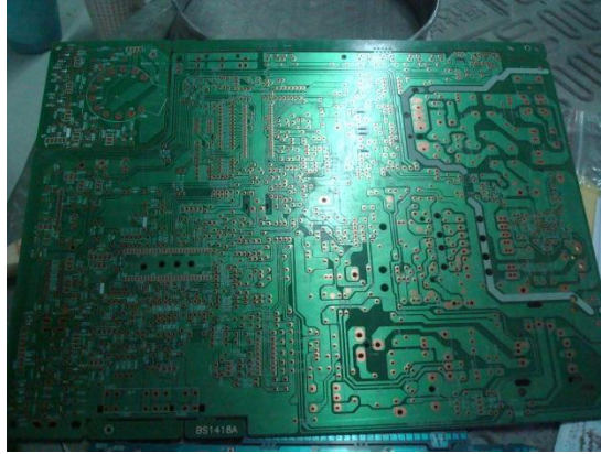
Figure 15: Waste printed circuit boards after toxic parts are removed
