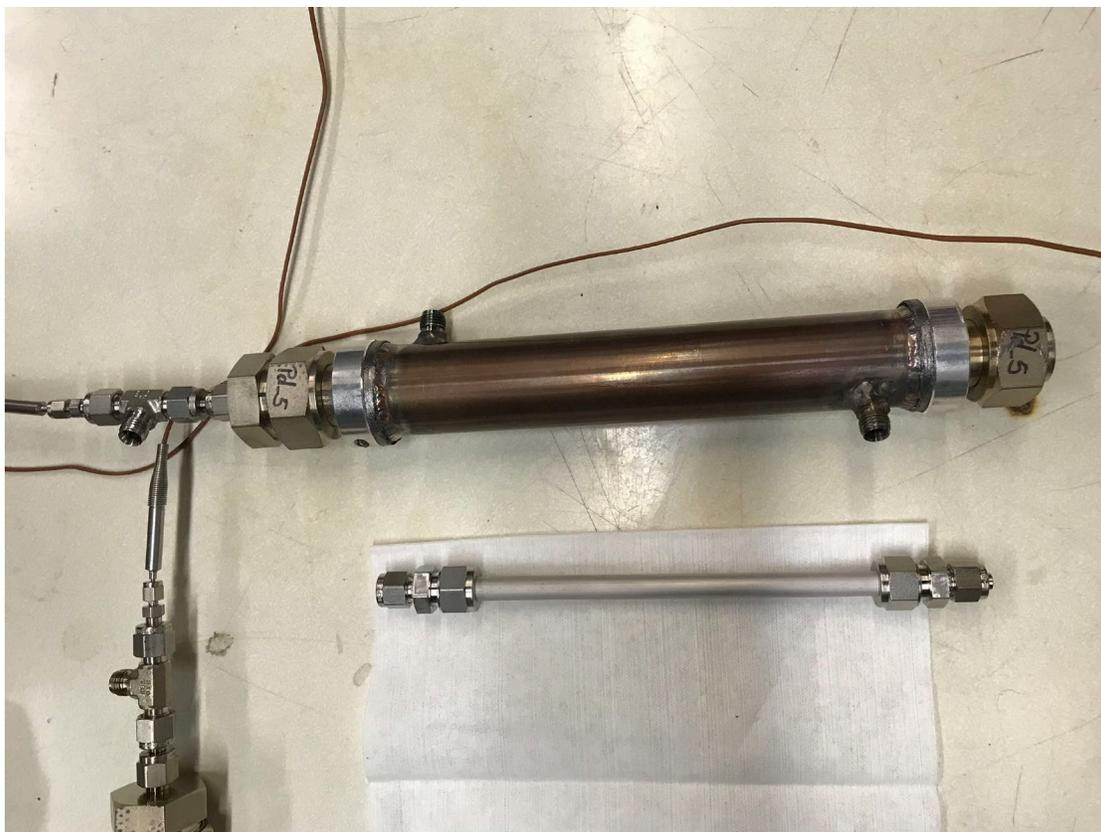
**Figure 3-3. Image of the Pd membrane and membrane module**
