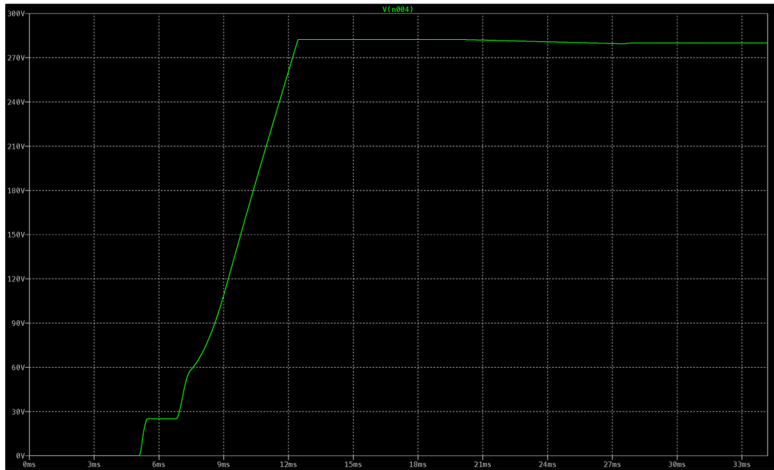
Figure F.65. Output voltage as a function of time for simulation test fourteen. At 12.5ms, the output voltage settled to 280V. Afterwards, at 20ms a resistor of 560 \Omega was applied to the output. From 30ms to 31ms, the input voltage transitioned from 50V to 100V.
