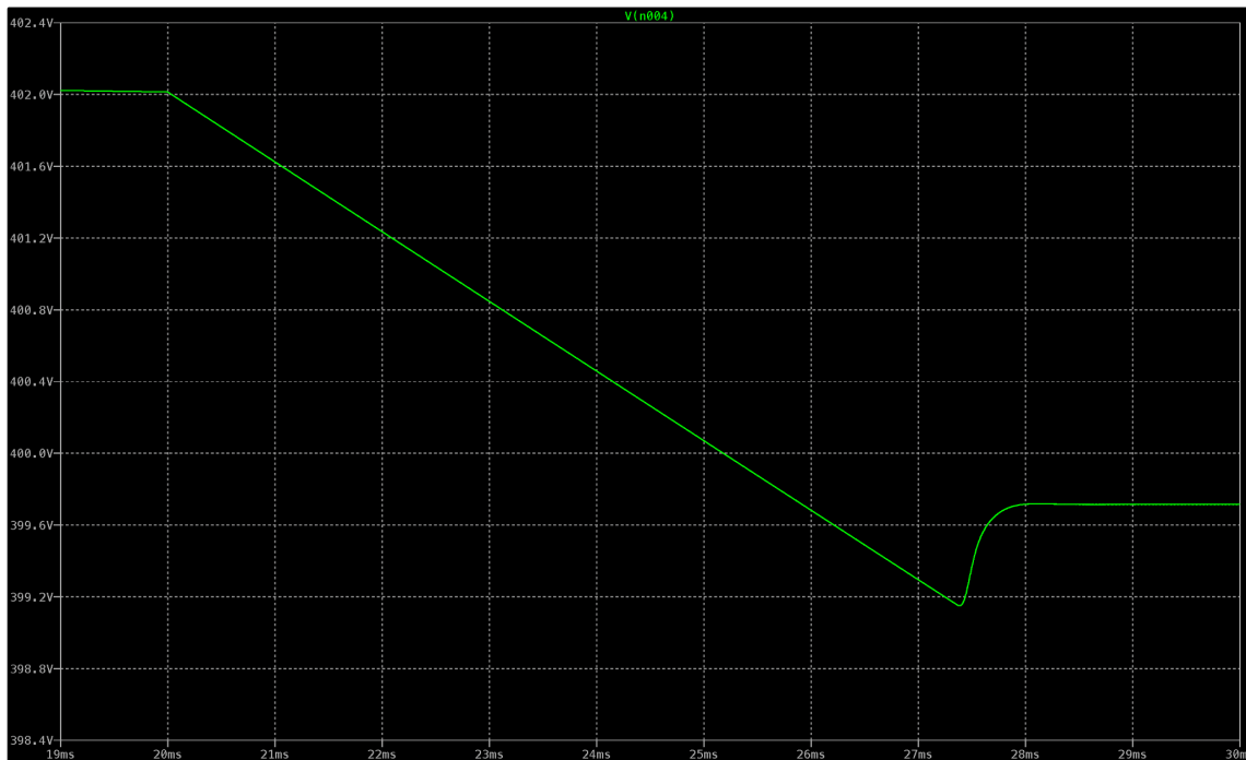
Figure F.30. Response to the application of the resistor of 800\Omega for simulation test six. The transients decayed after approximately 8ms. Additionally, the undershoot is about 600mV and the ripple once steady-state is achieved appears negligible.
