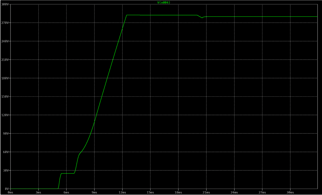
Figure F.62. Output voltage as a function of time for simulation test thirteen. At 12.5ms, the output voltage settled to 280V. Afterwards, at 20ms a resistor of 25.45\Omega was applied to the output. From 30ms to 31ms, the input voltage transitioned from 50V to 100V.
