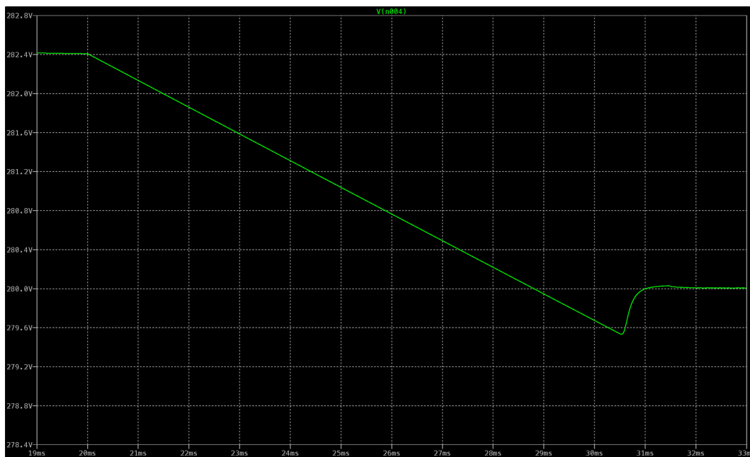
Figure F.40. Response to the application of the resistor of 800\Omega for simulation test eight. The transients decayed after approximately 12ms. Additionally, the undershoot is approximately 500mV and the ripple once steady-state is achieved appears negligible.
