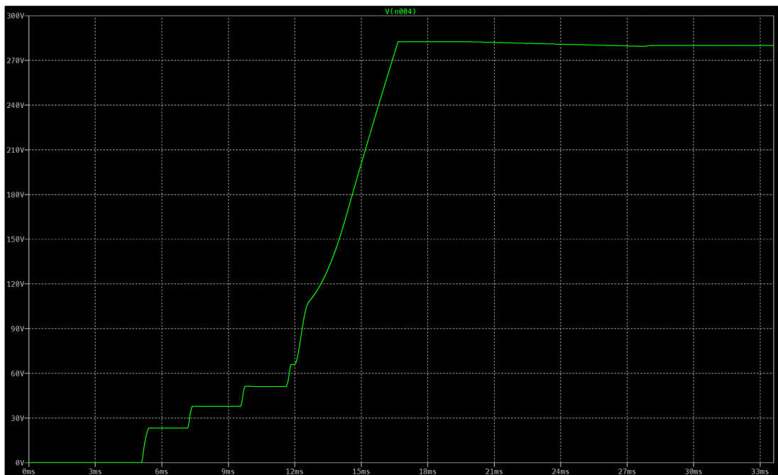
Figure F.69. Output voltage as a function of time for simulation test sixteen. At approximately 16ms, the output voltage settled to 280V. Afterwards, at 20ms a resistor of 560 \Omega was applied to the output. From 30ms to 31ms, the input voltage transitioned from 50V to 100V.
