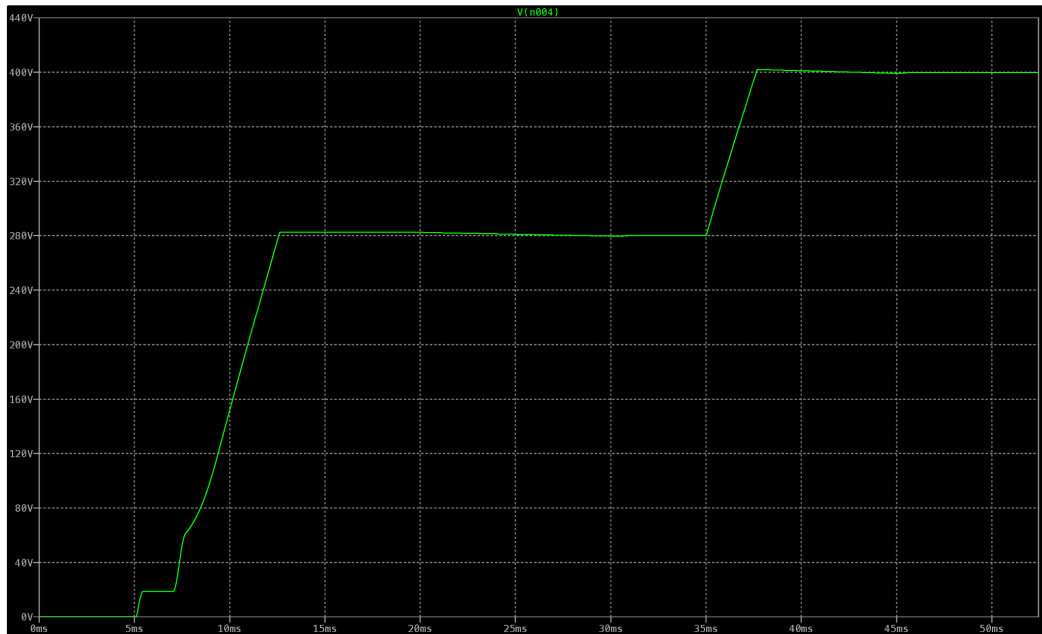
Figure F.39. Output voltage as a function of time for simulation test eight. At approximately 12.5ms, the output voltage settled to 280V. Afterwards, at 35ms a resistor of 800\Omega was applied to the output. Lastly, from 35ms to 38ms, the output voltage transitioned from 280V to 400V.
