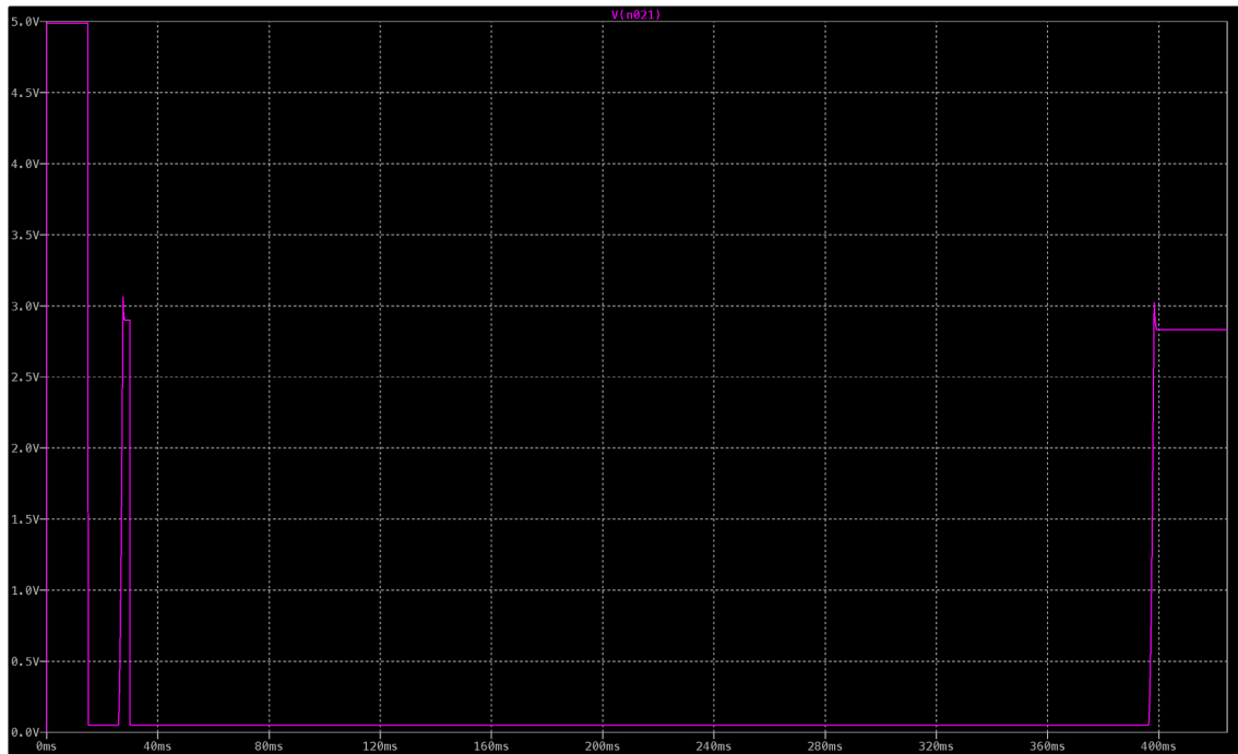
Figure F.32. Voltage waveform on the COMP pin with respect to ground for simulation test six. Compare this figure with Figure F.29 to discern what each non-zero voltage interval corresponds to.
