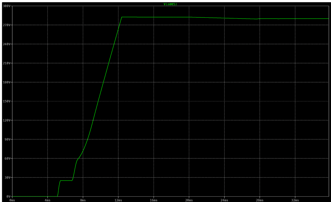
Figure F.19. Output voltage as a function of time for simulation test four. At approximately 12.5ms, the output voltage settled to 280V. Afterwards, at 20ms a 0.5A load was applied to the output. Lastly, at 30ms, the load transitioned from 0.5A to 11A.
