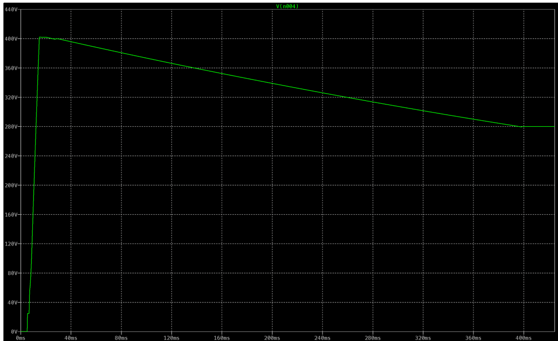
Figure F.29. Output voltage as a function of time for simulation test six. At approximately 15ms, the output voltage settled to 400V. Afterwards, at 30ms a resistor of 800\Omega was applied to the output. Lastly, from 30ms to 400ms, the output voltage transitioned from 400V to 280V.
