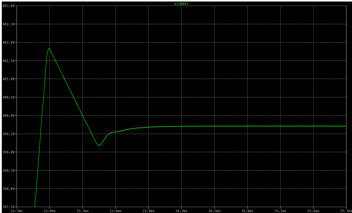
Figure F.36. Response to transitioning from 280V to 400V. When the output first attained 400V, the transients decayed after approximately 1.5ms. Additionally, the overshoot is about 2V and the ripple once steady-state is achieved appears negligible.
