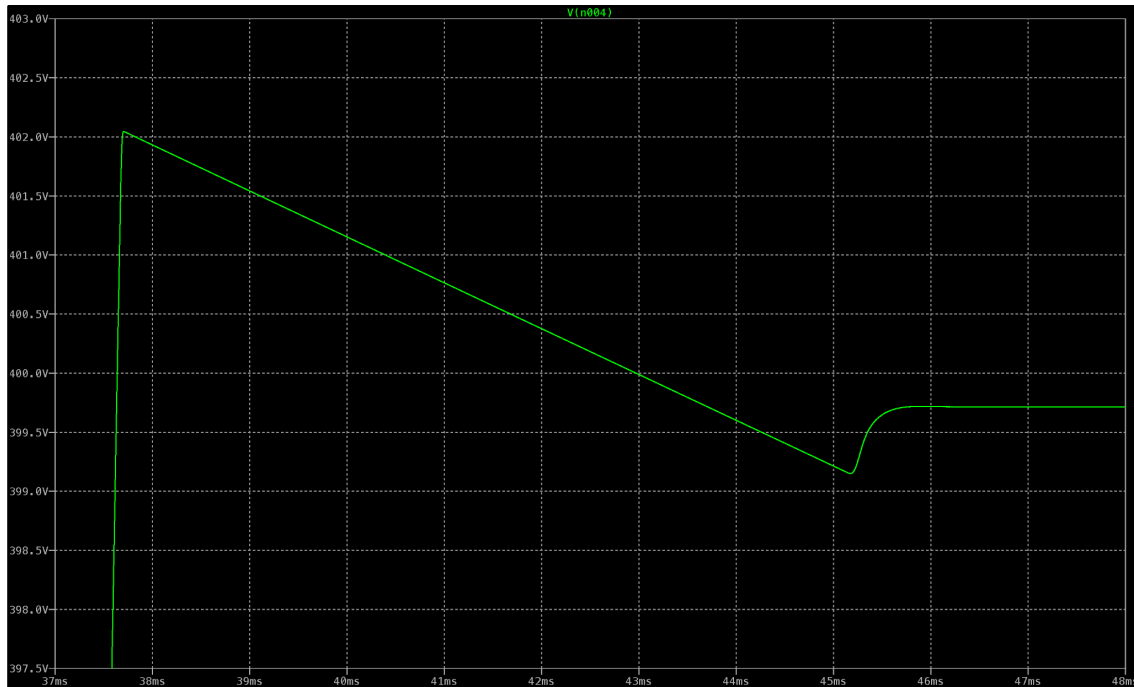
Figure F.41. Response to transitioning from 280V to 400V. When the output first attained 400V, the transients decayed after approximately 9ms. Additionally, the overshoot is about 2V and the ripple once steady-state is achieved appears negligible.
