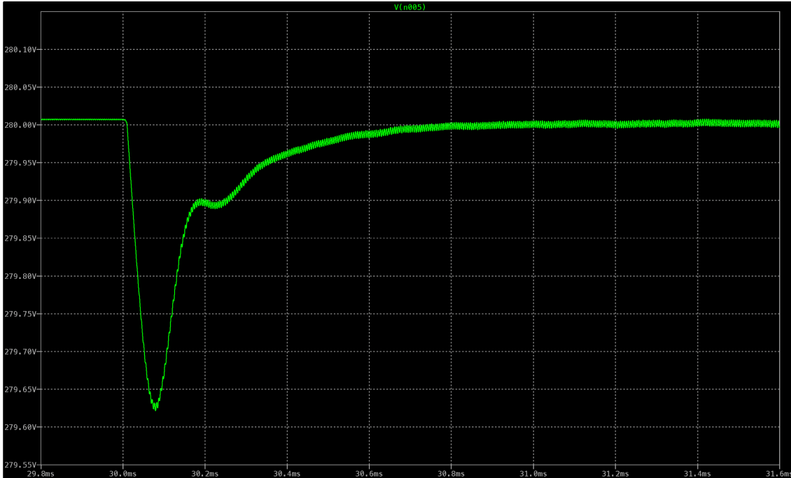
Figure F.21. Response to the application of the 11A load from 0.5A for simulation test four. The transients decayed after approximately 1ms. Additionally, the undershoot is nearly 400mV and the ripple once steady-state is achieved appears negligible.
