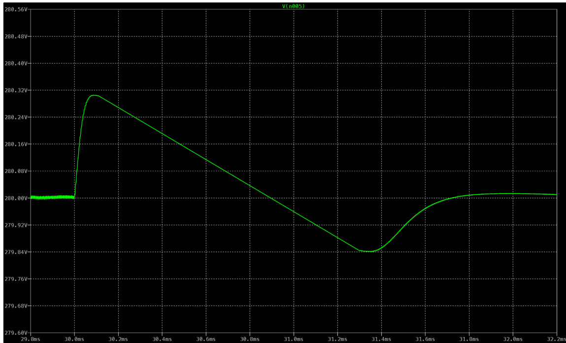
Figure F.16. Response to the application of the 0.5A load from 11A for simulation test three. The transients decayed after 2ms. Additionally, the overshoot is 300mV, undershoot 170mV, and the ripple once steady-state is achieved appears negligible.
