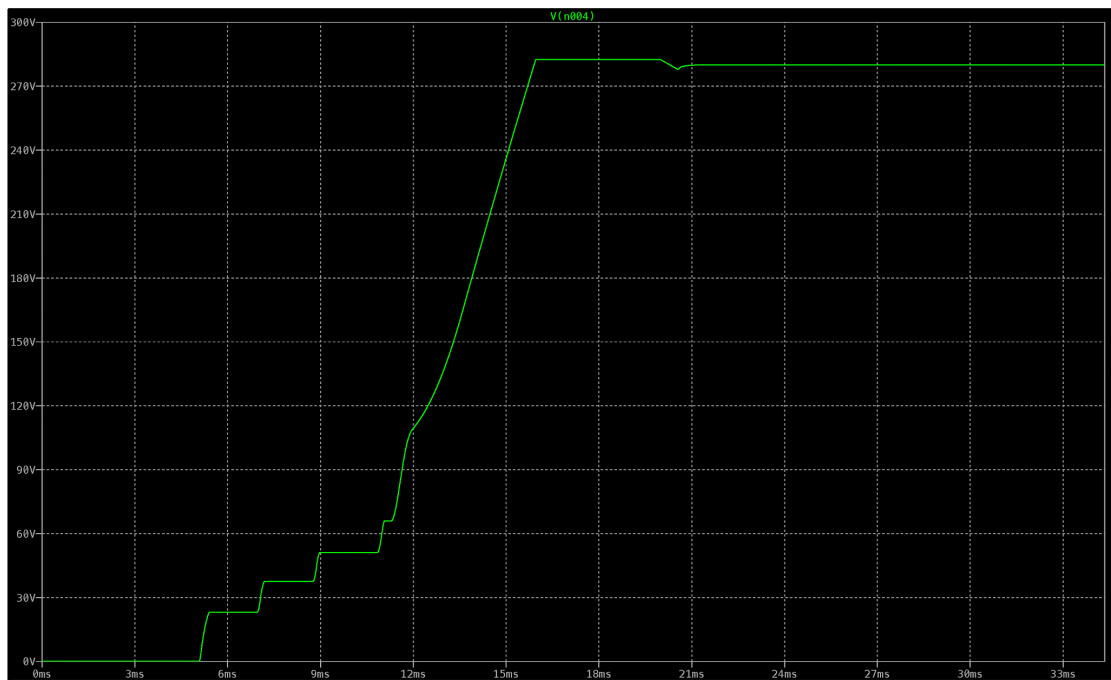
Figure F.67. Output voltage as a function of time for simulation test fifteen. At approximately 16ms, the output voltage settled to 280V. Afterwards, at 20ms a resistor of 25.45\Omega was applied to the output. From 30ms to 31ms, the input voltage transitioned from 100V to 50V.
