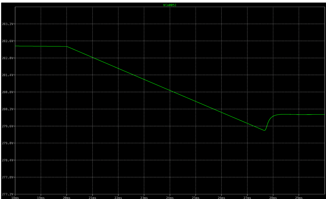
Figure F.20. Response to the application of the 0.5A load from 0A for simulation test four. The transients decayed after approximately 9ms. Additionally, the undershoot is about 600mV and the ripple once steady-state is achieved appears negligible.
