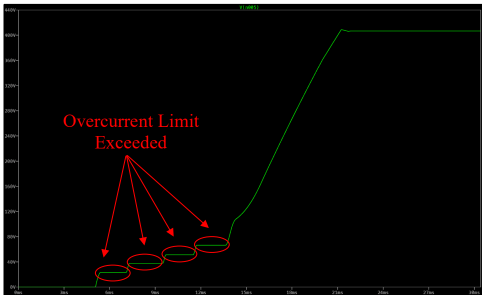
Figure 7.8. Simulation displaying excession of the overcurrent limit four times from 5.5ms to 14ms at an input voltage of 100VDC. Each time the overcurrent limit is exceeded, the soft-start capacitor recharges to its value before the overcurrent limit was exceeded, creating a sawtooth waveform on the SS pin from 5.5ms to 14ms.
