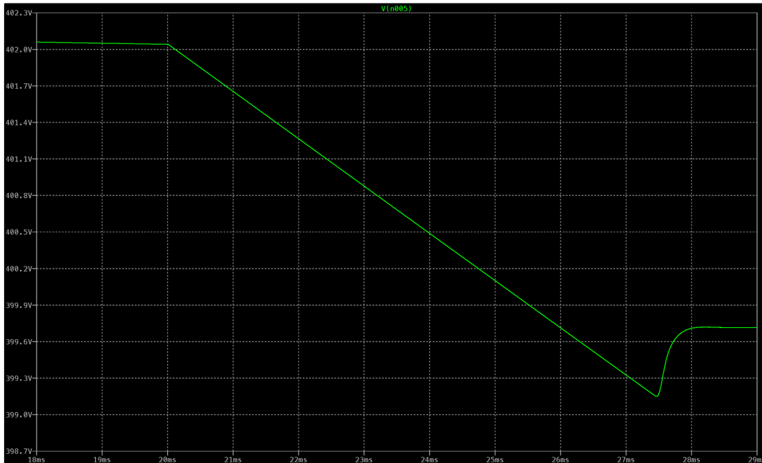
Figure F.10. Response to the application of the 0.5A load from 0A for simulation test two. The transients decayed after approximately 8ms. Additionally, the undershoot is nearly 600mV and the ripple once steady-state is achieved appears negligible.
