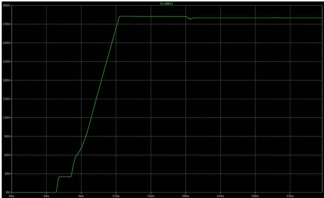
Figure F.14. Output voltage as a function of time for simulation test three. At approximately 12.5ms, the output voltage settled to 280V. Afterwards, at 20ms an 11A load was applied to the output. Lastly, at 30ms, the load transitioned from 11A to 0.5A.
