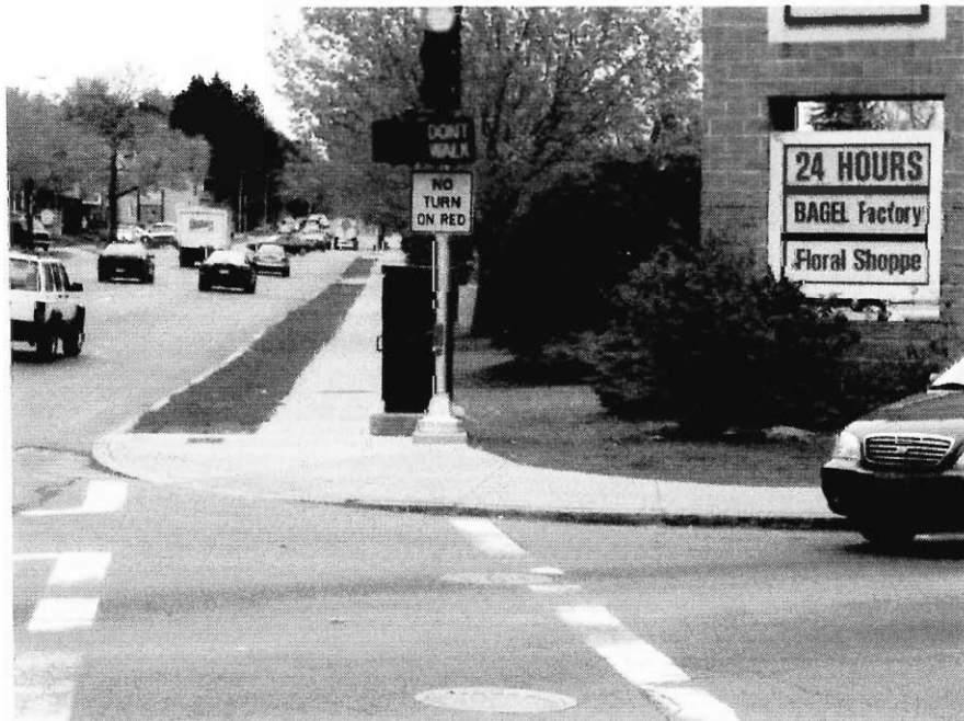
Figure 12 - Sharp right turn, observe tire marks on the sidewalk
