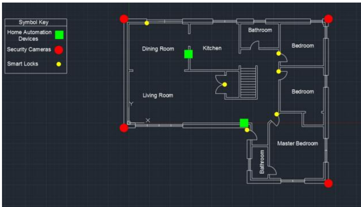
Figure 17. AutoCAD First Floor Plan with Devices
