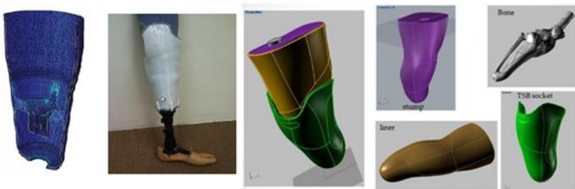
Figure 28: 3D Printed Socket Creation Process 65
