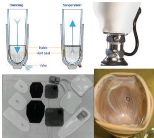
Figure 26: Vacuum suspension socket 56 and Inflatable bladders 57
