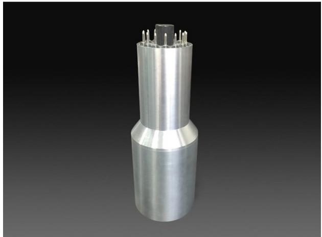
Figure 2.8.: 3x3 Sodium Iodide crystal
