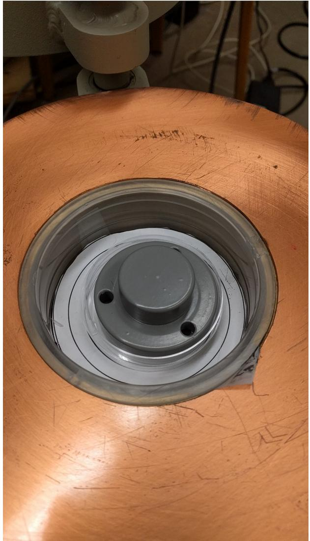
Figure 2.2.: Simulated loaded petri dish with lead weight placed in detector
