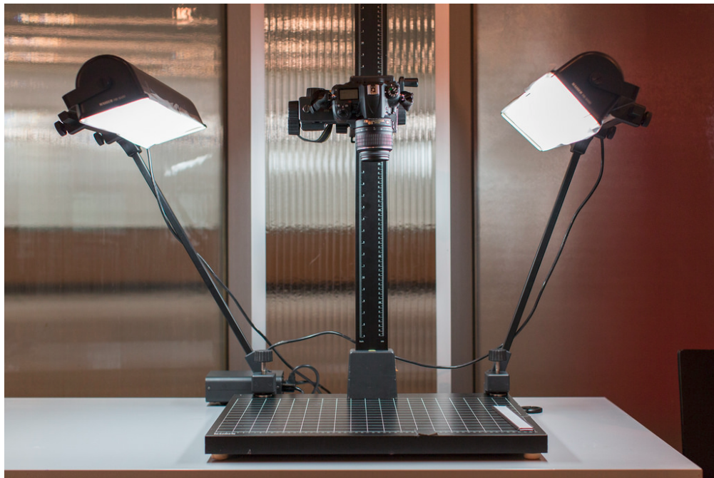
Figure 6: A copy stand for document digitization Licensed under Creative Commons Attribution 2.0 Generic License
