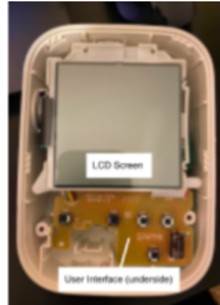
15B: OMRON Blood Pressure Monitor Interior User Interface Surface with Removal of Cover
