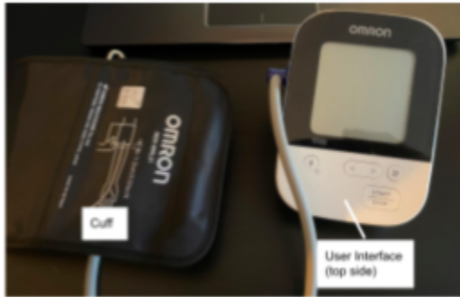
15A: OMRON Blood Pressure Cuff Exterior and User Interface
