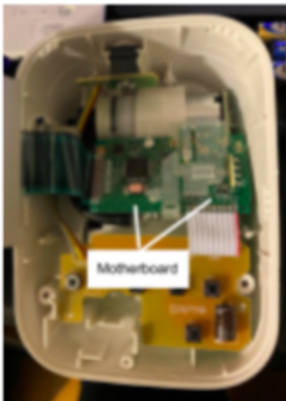
15C: OMRON Blood Pressure Monitor Motherboard with a View of Mini Pump
