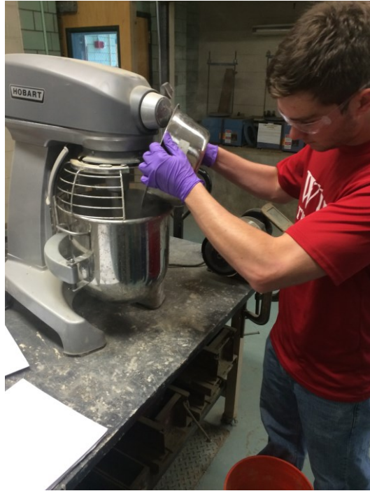
Figure 6 Materials being added to mixer
