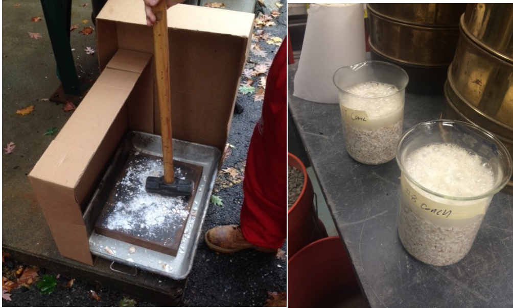
Figure 5 Shells being tamped to correct size and undergoing acid treatment
