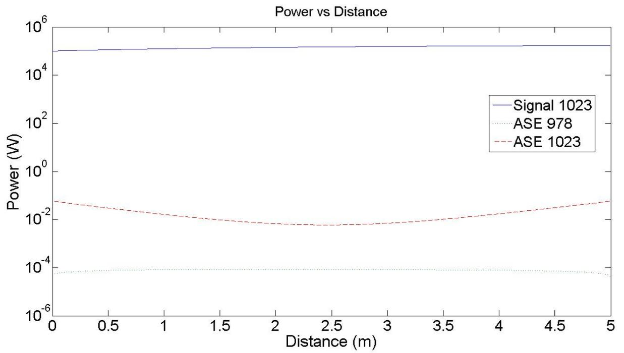
Figure 41: Signal, 978 and 1023 nm ASE Power vs Distance,  $P_s = 10^4$  W,  $P_p = 10^5$  W
