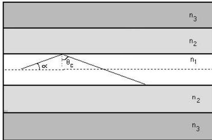
Figure 2: Double Cladding Fiber
