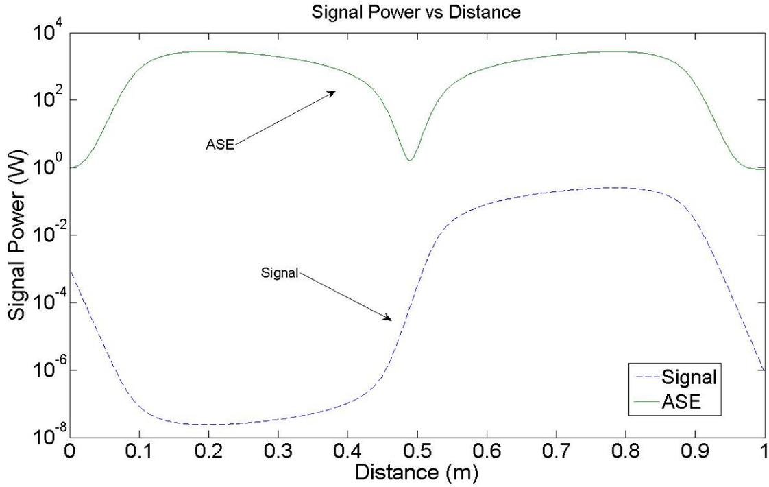
Figure 49: Signal and 978 nm ASE Powers vs Distance for 1 m
