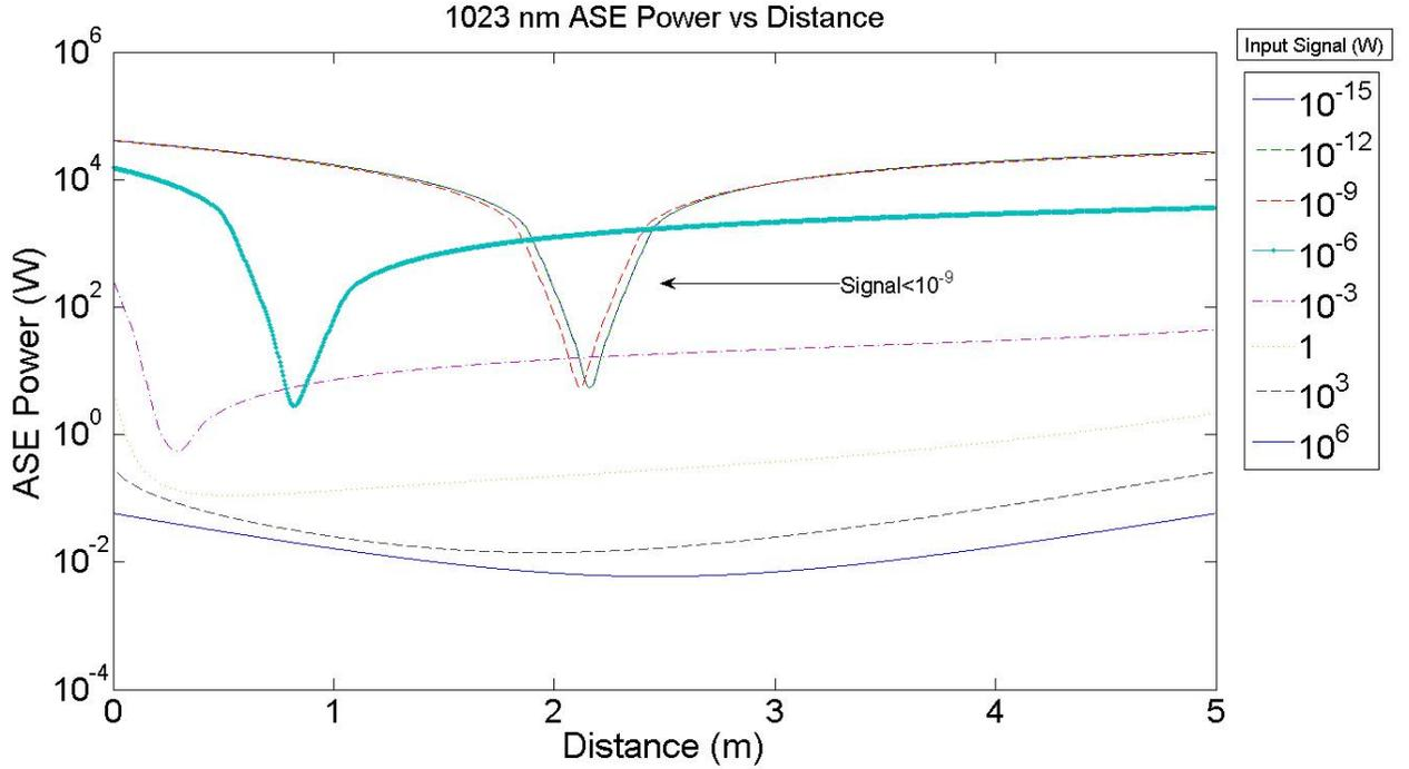
Figure 35: 1023 nm ASE vs Distance,  $P_p 10^5$  W
