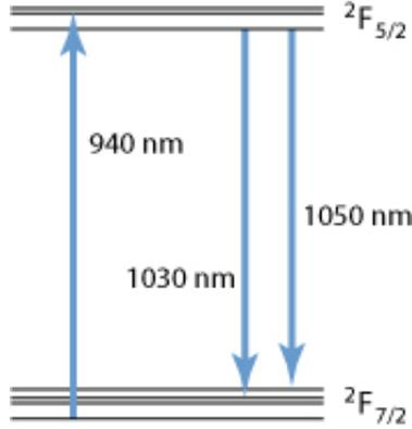
Figure 32: Energy Level Diagram for Yb
