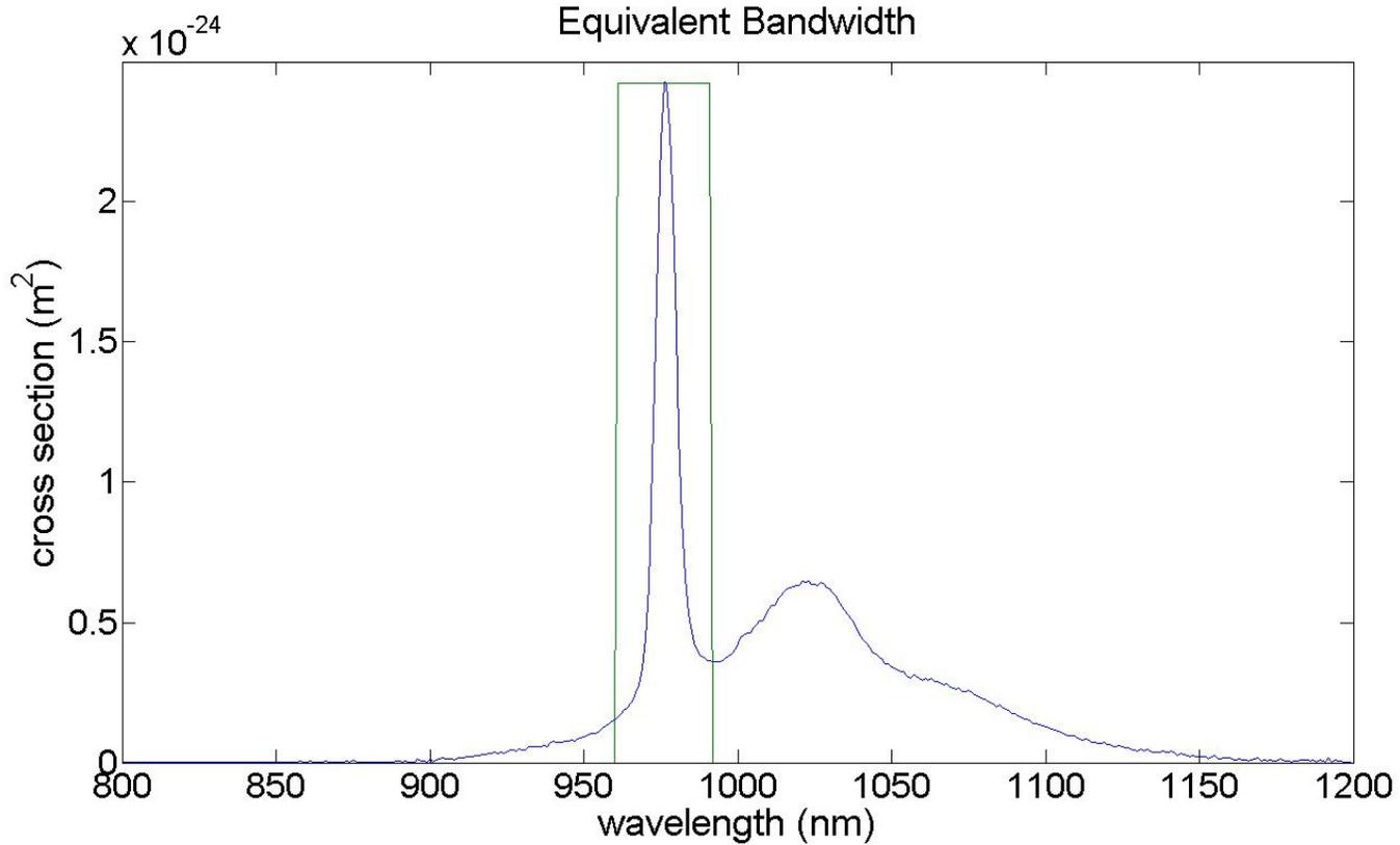
Figure 13: Emission Cross Section Spectrum with Equivalent ASE Band, One Bin
