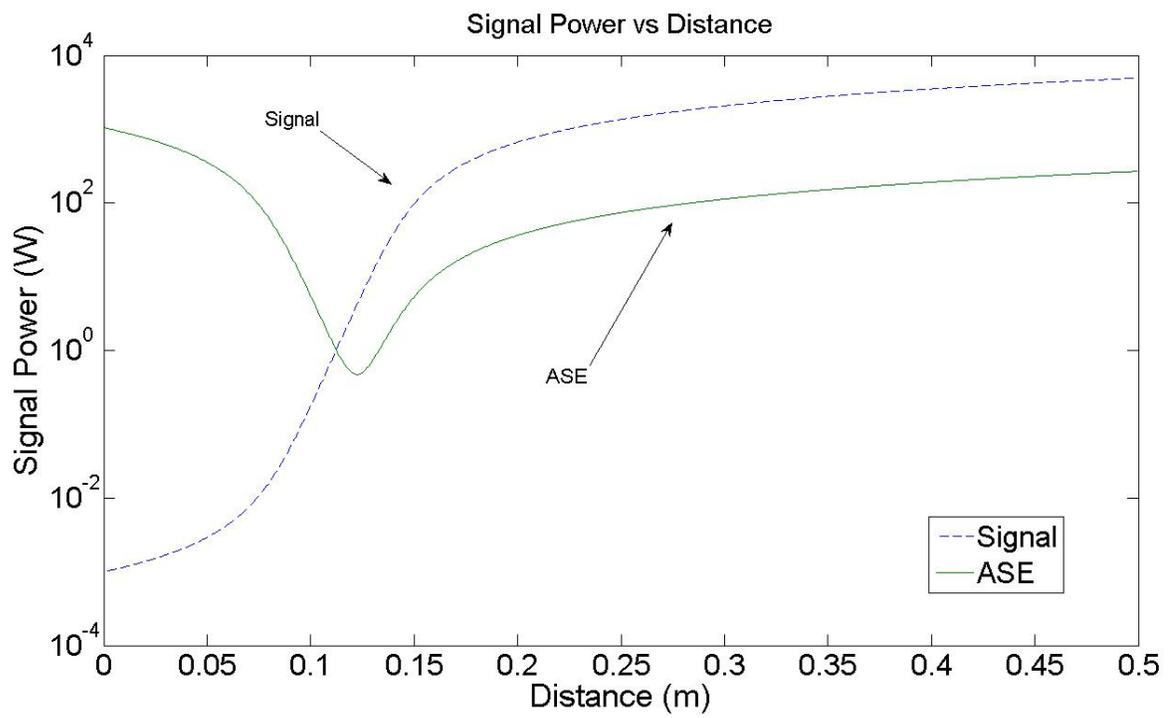
Figure 50: Signal and 978 nm ASE Powers vs Distance for 50 cm
