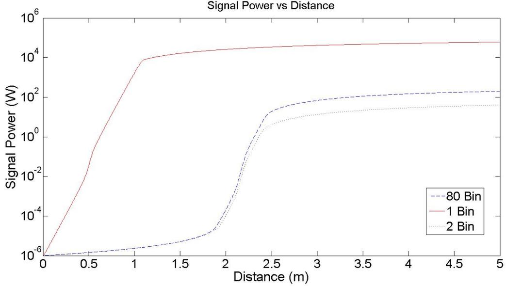
Figure 25: Signal Power vs Distance for 1, 2, and 80 bin ASE Models
