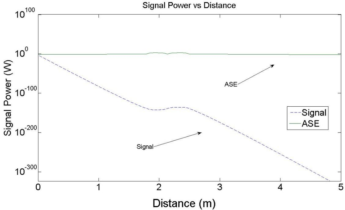
Figure 48: Signal and 978 nm ASE Powers vs Distance for 5 m
