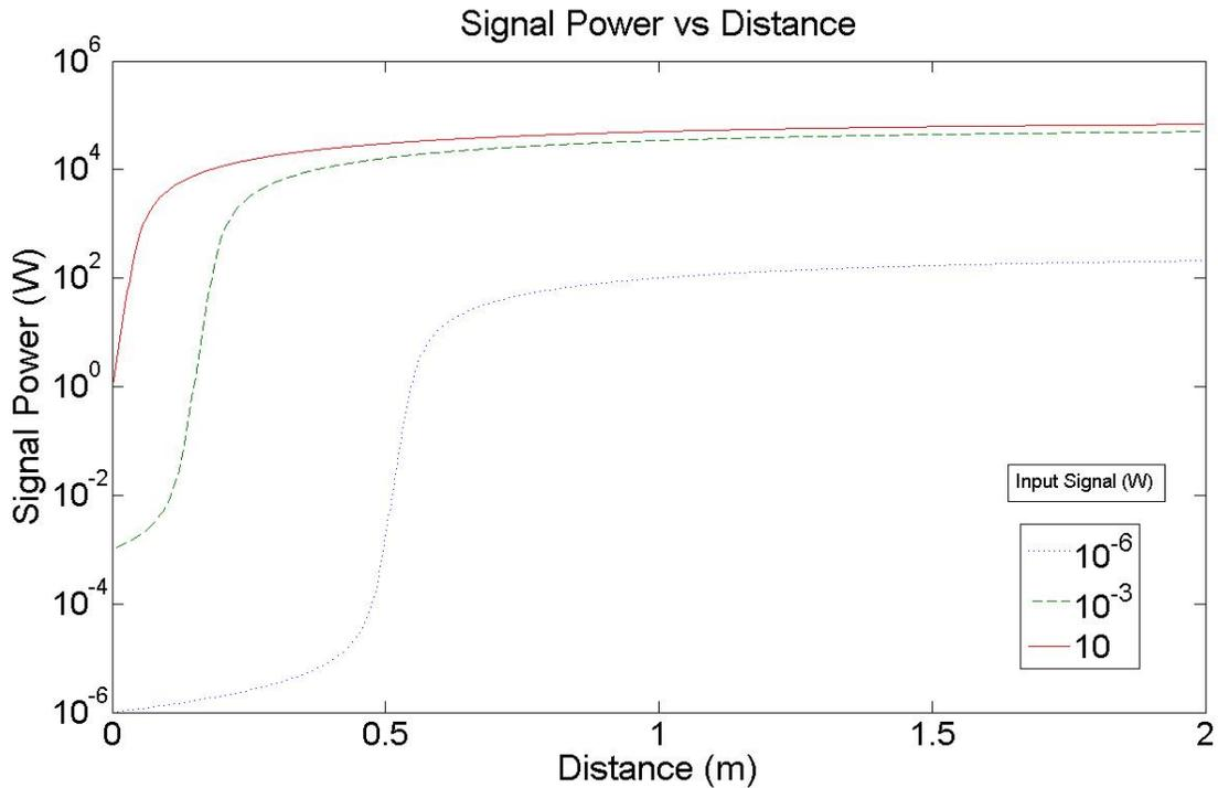
Figure 69: Signal vs Distance, 1060 nm Signal,  $P_p = 10^5$  W
