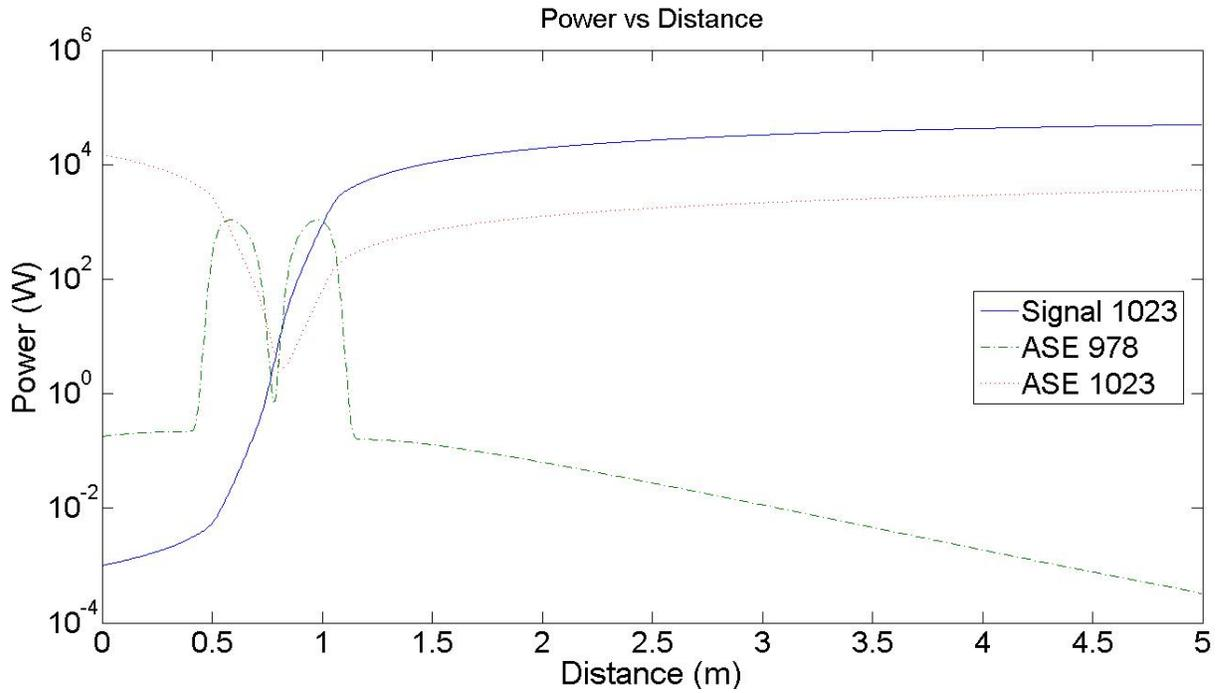
Figure 37: Signal, 978 and 1023 nm ASE Powers vs Distance,  $P_s = 10^{-3}$  W,  $P_p = 10^5$  W
