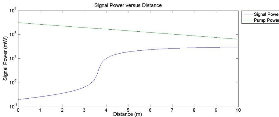
Figure 20: Signal and Pump Powers, Two Bin ASE Model
