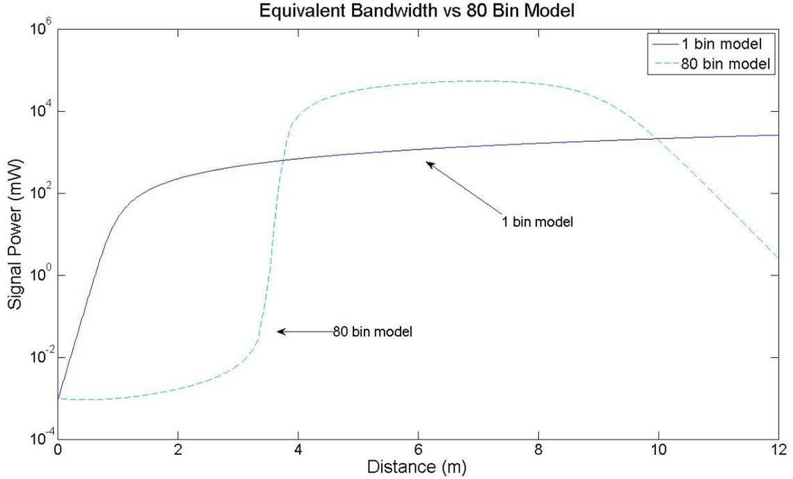
Figure 17: One Bin versus Integrated ASE Model for 12 m, Signal at 1023 nm and  $P_s = 10^{-3}$  W
