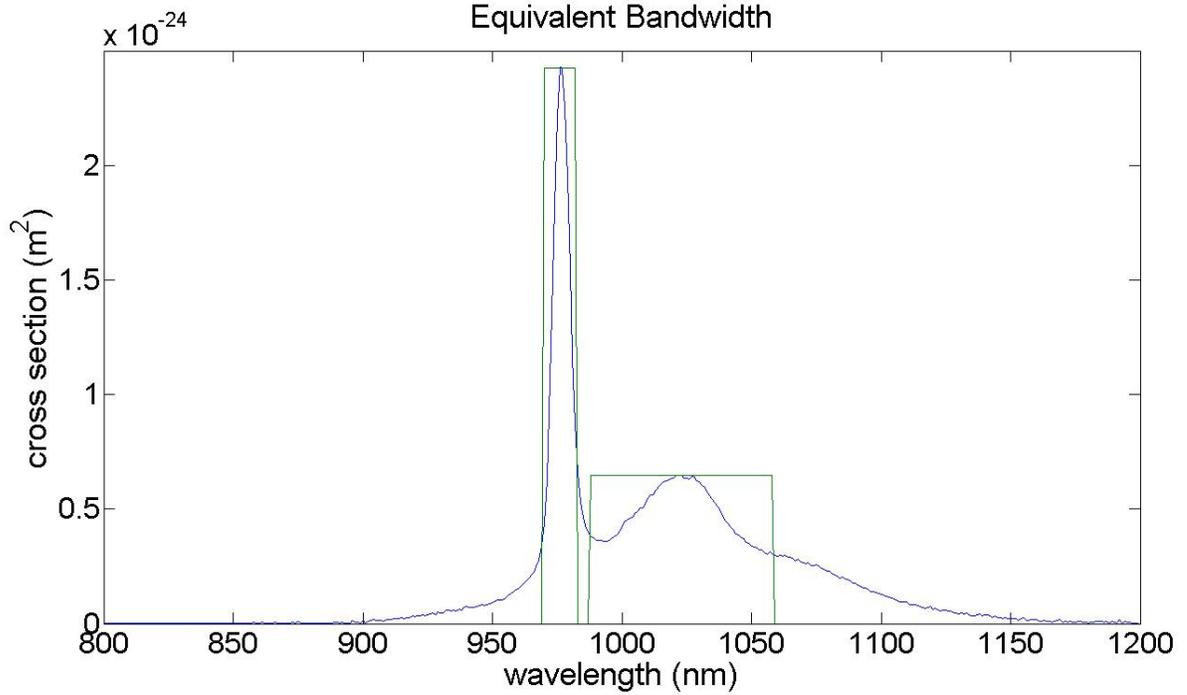
Figure 18: Emission Cross Section Spectrum with Equivalent ASE Band, Two Bin
