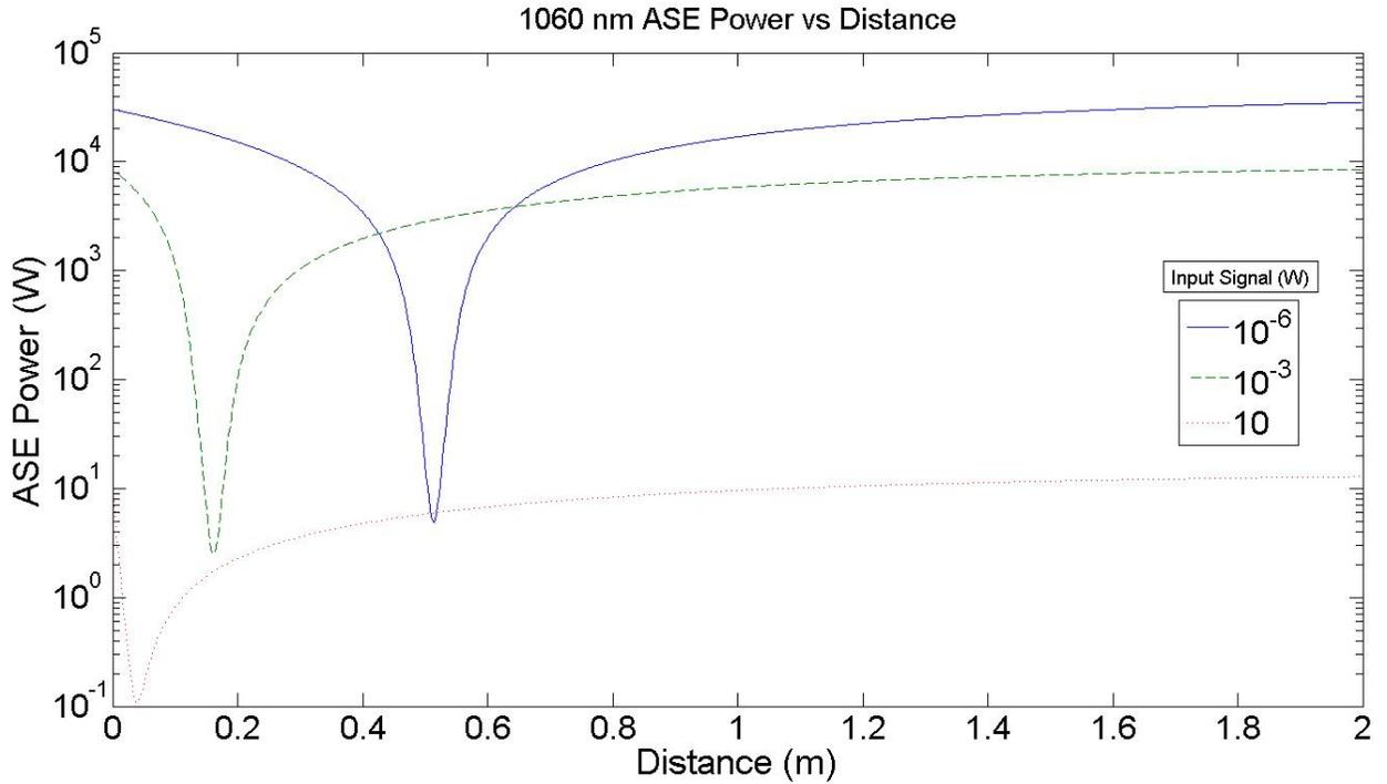
Figure 70: 1060 nm ASE vs Distance, Signal at 1060 nm,  $P_p = 10^5$  W
