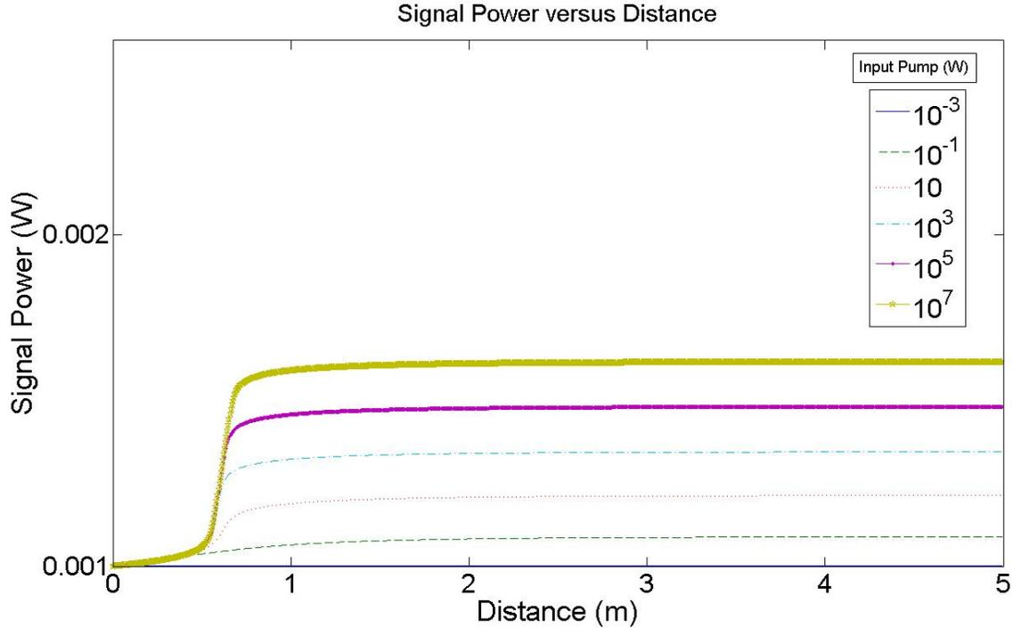
Figure 64: Signal Power vs Distance,  $P_s = 10^{-3}$  W, Varied Pump, 1060 ASE included
