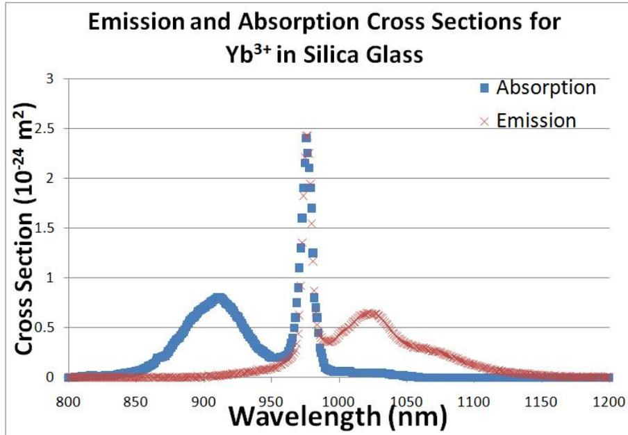
Figure 31: emission and absorption cross section for Yb
