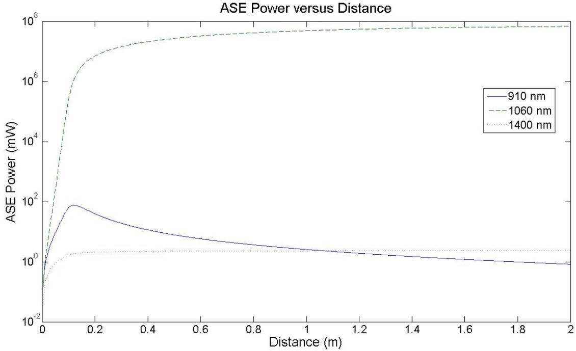
Figure 56: 910, 1060, and 1400 nm ASE, No Input Signal,  $P_p = 10^5$  W
