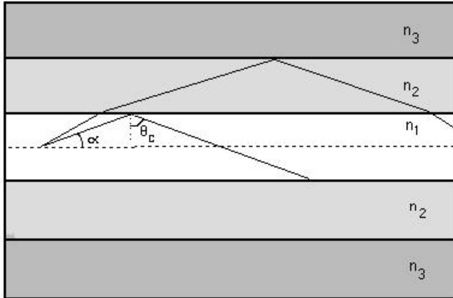
Figure 12: ASE trapped in cladding
