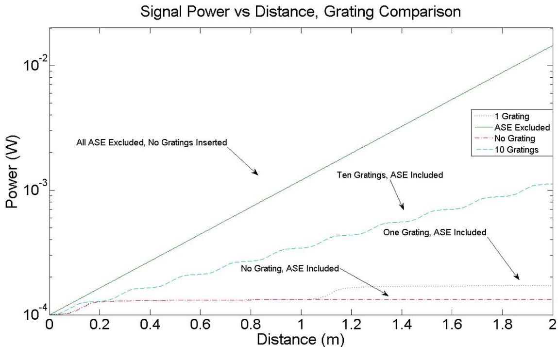
Figure 72: Signal Power vs Distance with Insertion of Diffraction Gratings,  $P_p = 10^3$  W and  $P_s = 10^{-4}$  W
