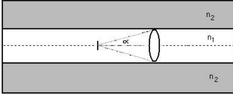
Figure 10: Solid Angle Trapped in Fiber
