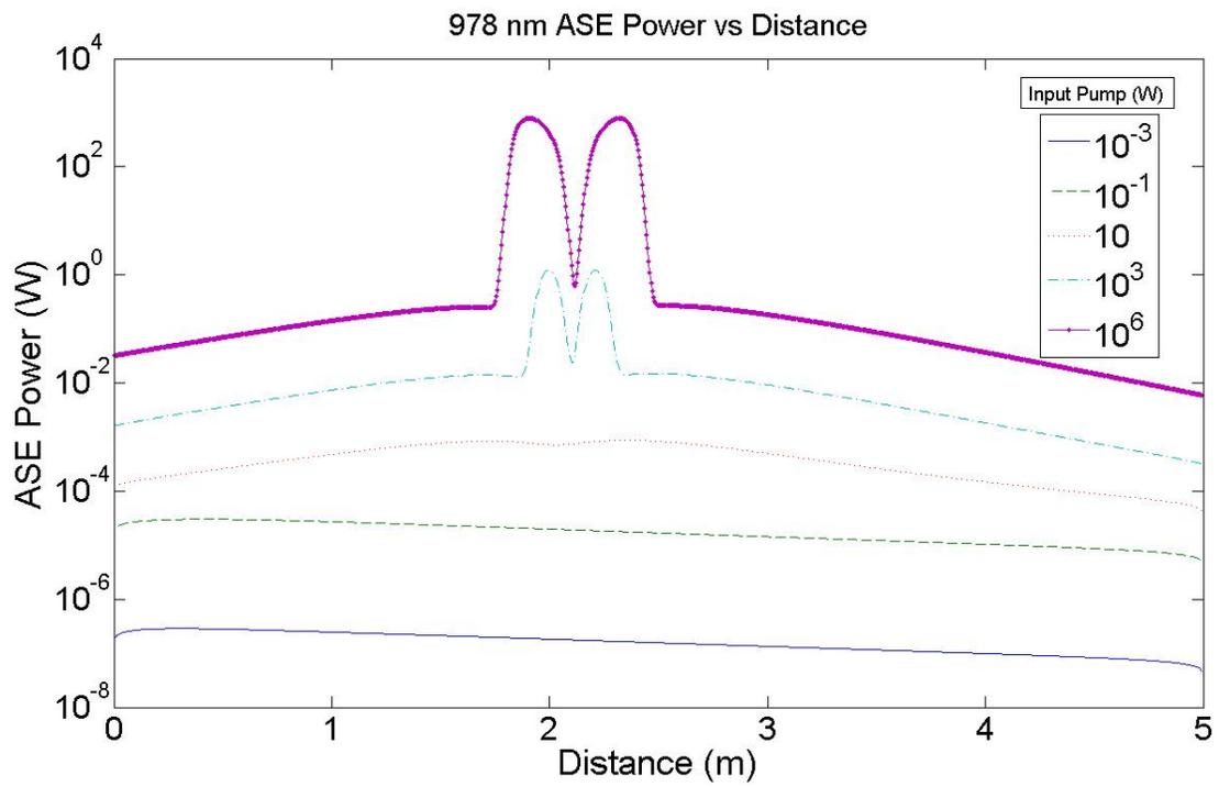
Figure 45: 978 nm ASE Power vs Distance,  $P_s = 10^{-5}$  W, Varied Pump
