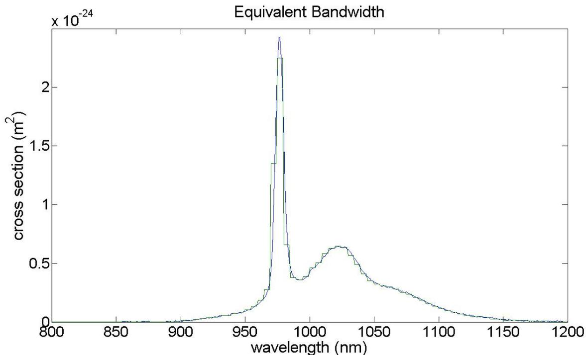
Figure 19: Emission Cross Section Spectrum with Equivalent ASE Band, 80 Bin
