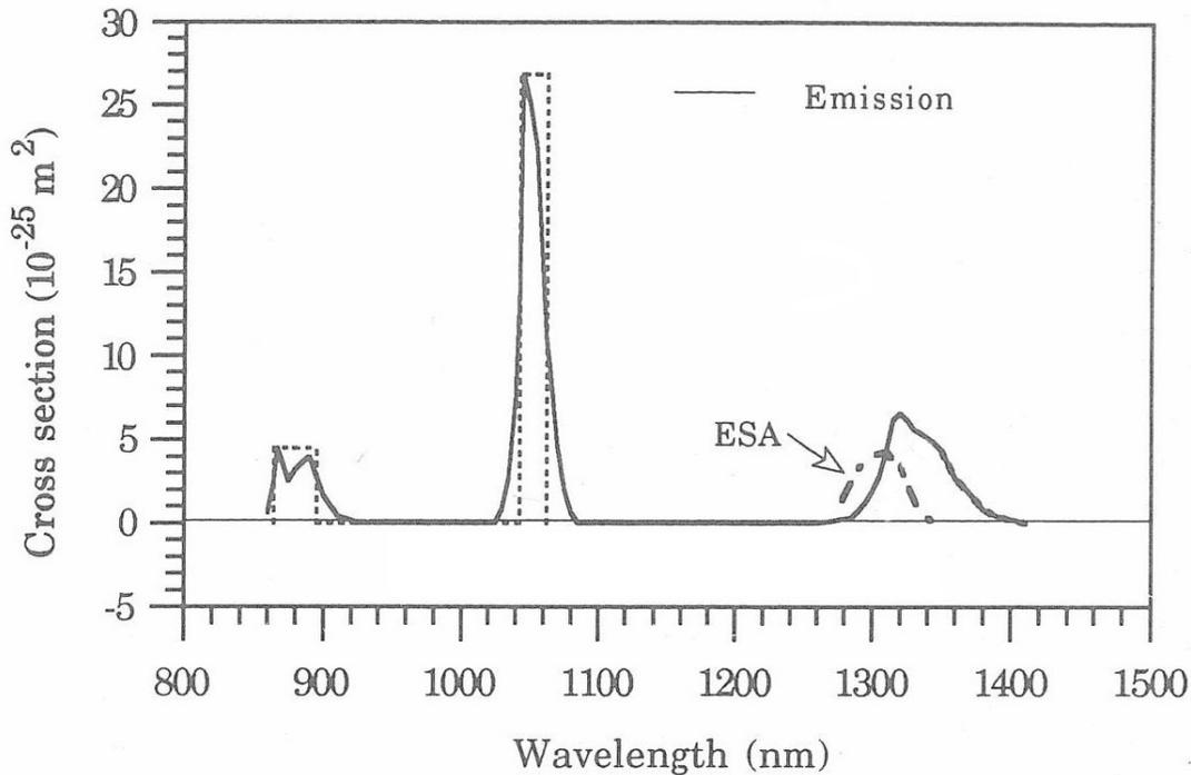
Figure 8: ESA Spectrum Shifted Relative to Spectrum in Silica, shown in Fluoride Host Glass.
