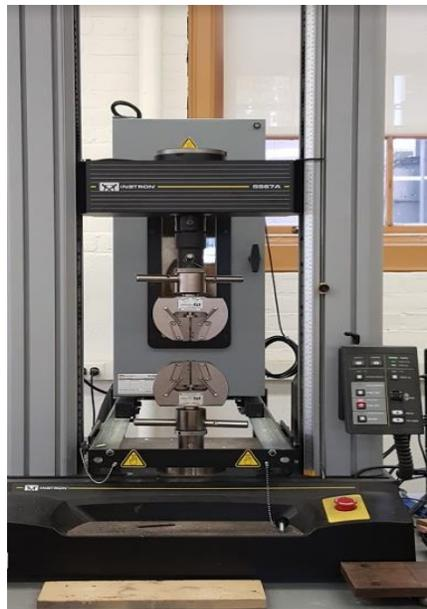
*Figure 14: The Instron 5567A was used for tensile testing.*
