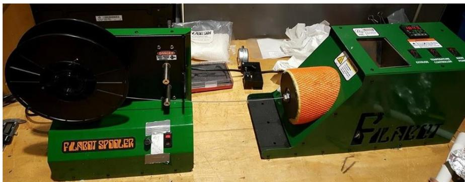
Figure 10: The Filabot extruder and spooler working together to produce filament.
