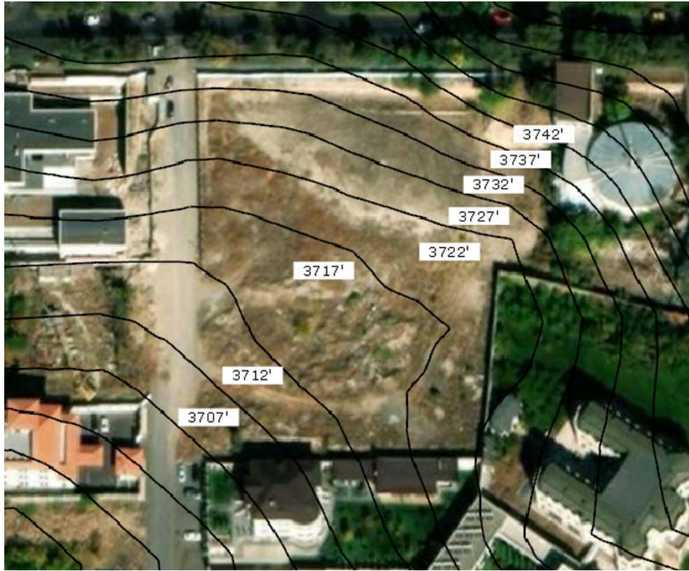
Figure 3.2: Contour Lines on Site Location
