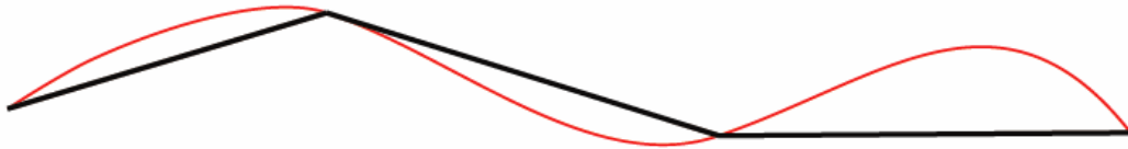
Figure 3.7: Spline Approximation Red curve is the spline which has been roughly approximated by assuming just two values of 0 and 1 as for its parameter.
