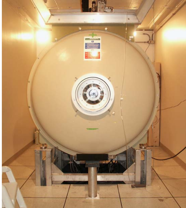
Figure 6.6: Bruker Biospec 4.7T/40cm horizontal magnet (Oxford Instruments, U.K.) equipped with a Biospec Bruker console (Bruker, MA, U.S.A) and a 20-G/cm magnetic field gradient insert.
