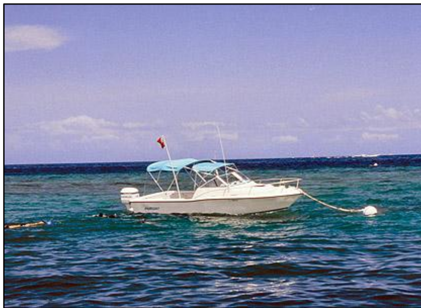
Figure 11: The correct way a boat latches onto a simple-structured mooring buoy (National Park Service, 2014).
