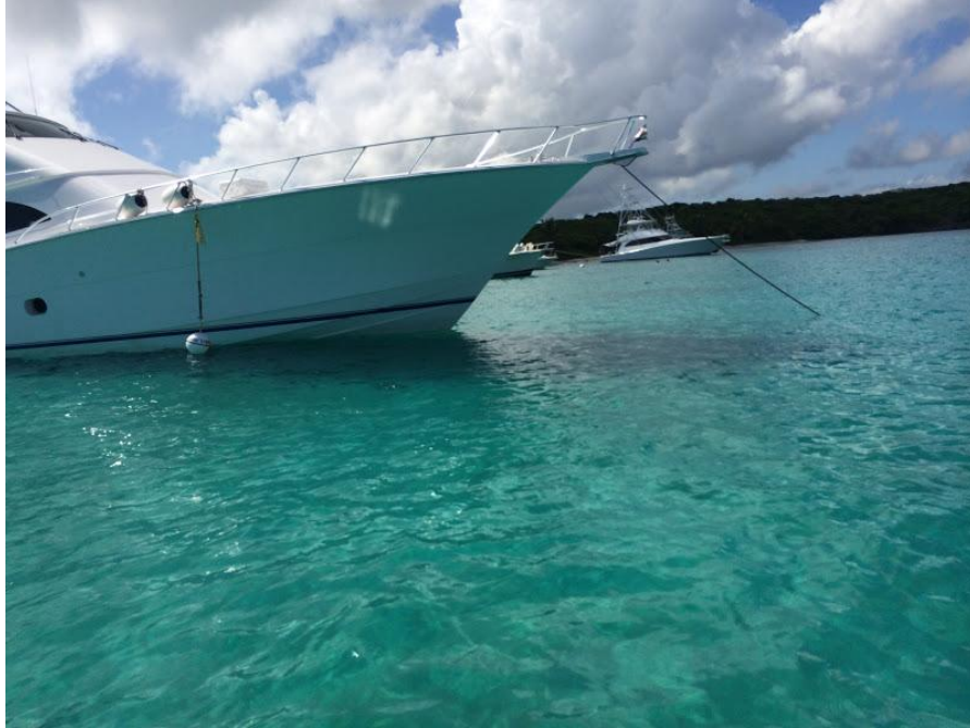
Figure 30: A boat attached to a mooring buoy and anchored at the same time
