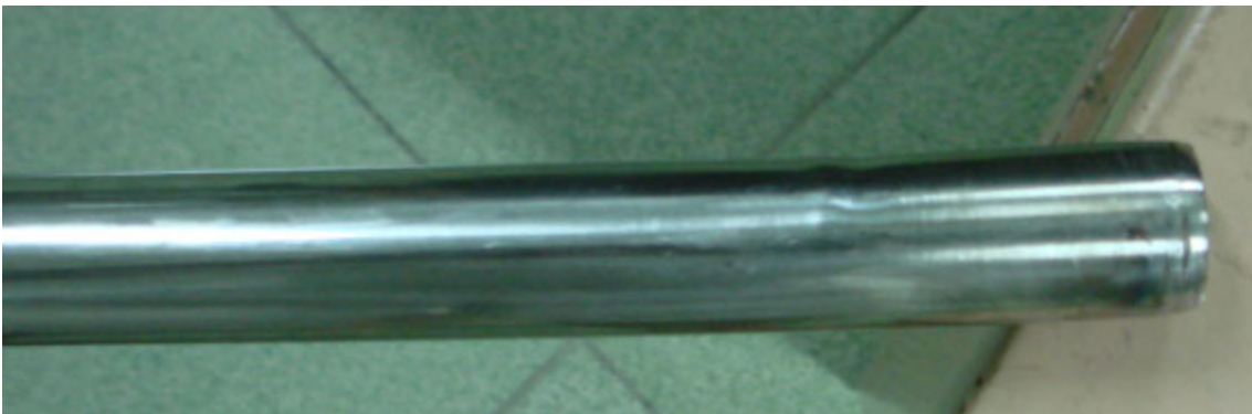
Figure 24: Bent lower pole
