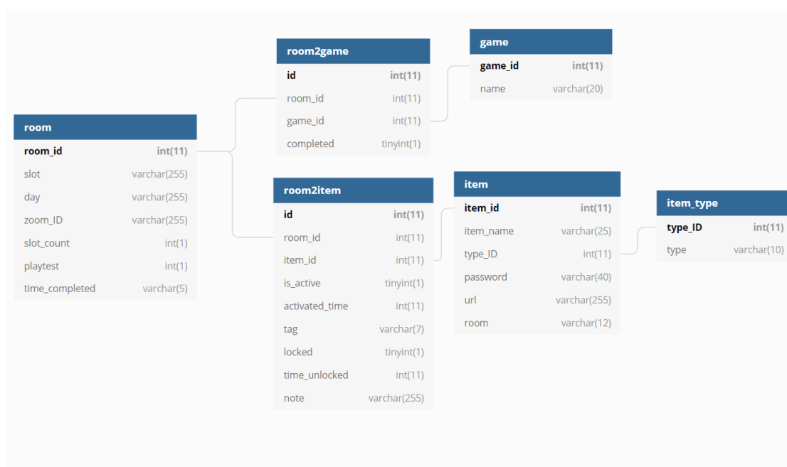
Figure 5.9: The tables containing the game data and analytics information for the experience (created using https://dbdiagram.io/d )
