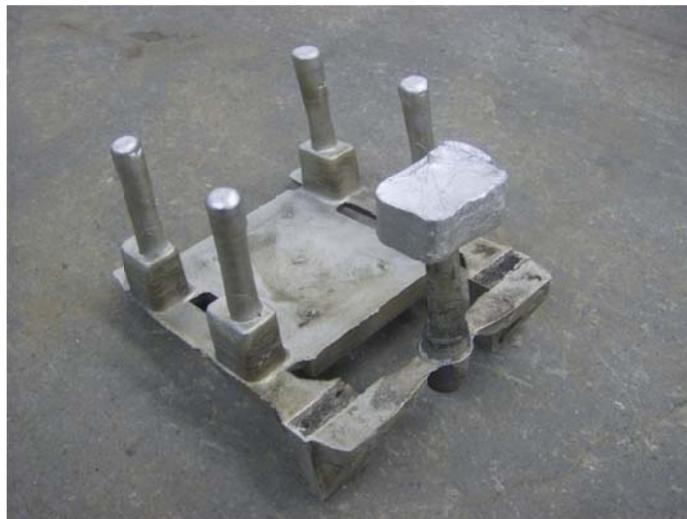
**Fig. 15** The complete casting.
