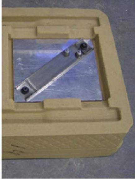
**Fig. A-2** Aluminum plate and strip heater assembly placed in mold cavity.
