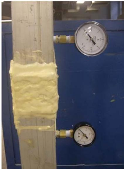
**Fig. C-1** Apparatus for measuring specific permeability of sand mold.
