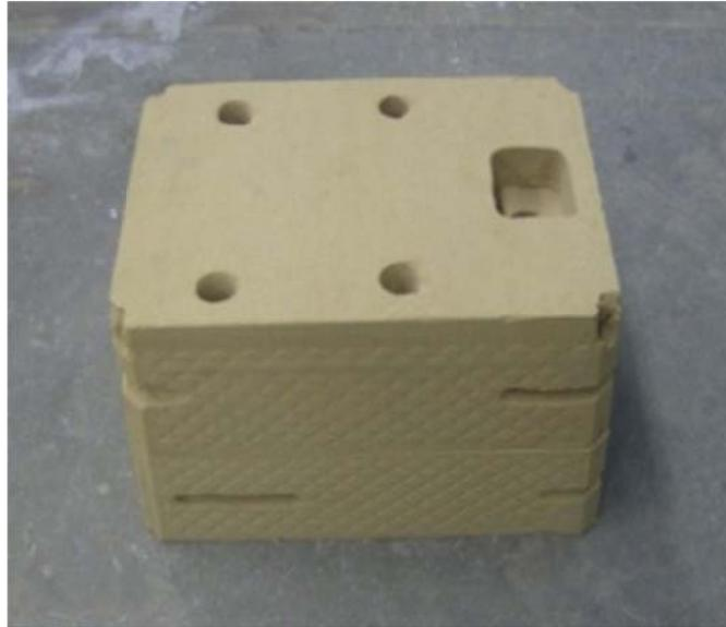
**Fig. 12** The sand mold used in the experiments.
