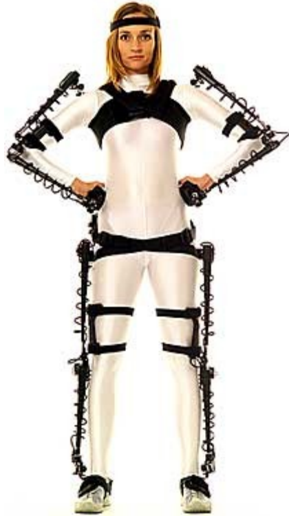
Figure IB1.4: An example of an "exoskeleton" motion capture suit.
