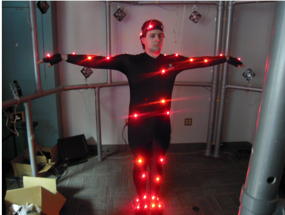
Figure IB1.2: WPI's motion capture suit when activated.
