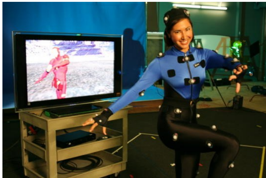
Figure IB1.1: An example of a “passive” suit.
