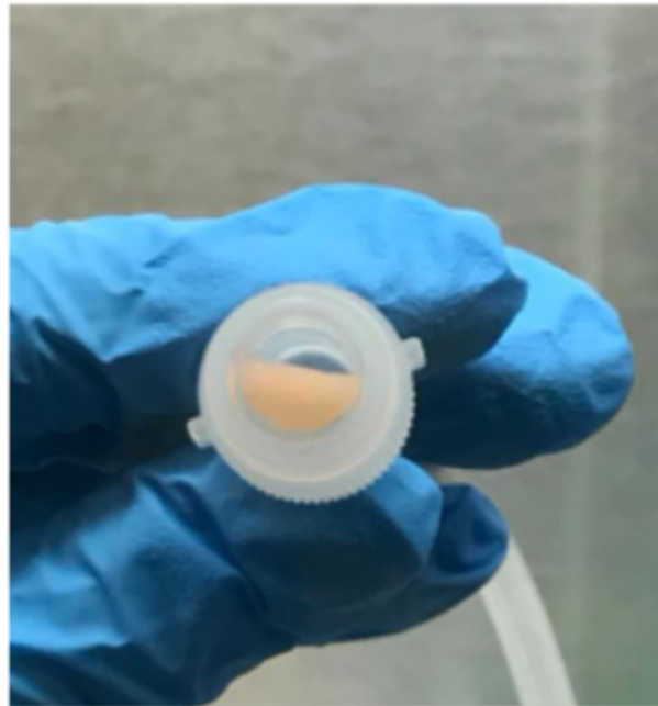
Figure 15: 10% silk scaffold cut to a half-moon with endothelial cells seeded on it. The scaffold is inserted into the 2 mm thick PDMS ring, which is then inserted into the Swinnex [23]
