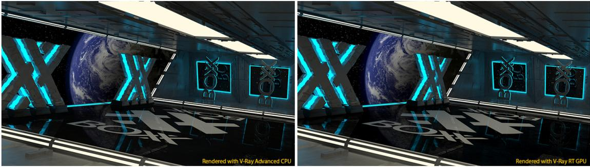
Figure 1: The left picture is rendered by CPU and the right one is by GPU. It's hard to tell the difference between them, but the GPU takes less time to render the graphic in comparison to the CPU. Figure taken from [11].
