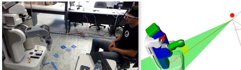
Figure 3.5: Example of our framework generating legible motions in response to human attention
