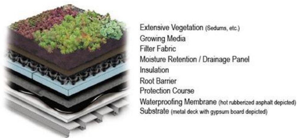
Figure 8 - Extensive Roof Section (Miller, 2011)
