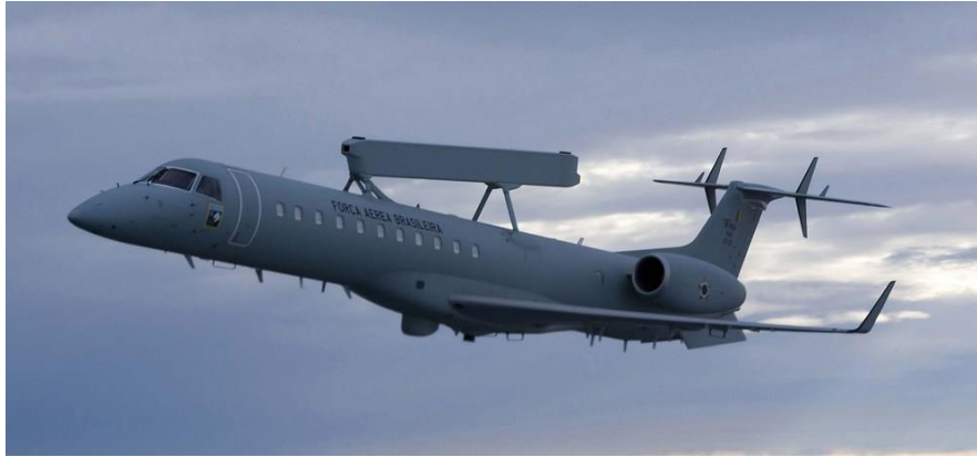
Figure 89. One-Dimensional phased array radar mounted on an airplane([Image of one-dimensional phased array], 2012).
