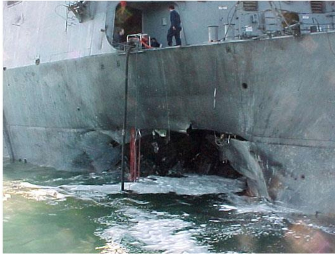
Figure 1. Damage to USS Cole after small craft bombing ([Image of USS Cole], 2012).
