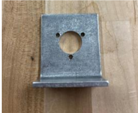
FIGURE 3.36 MILL MACHINED L BRACKETS
