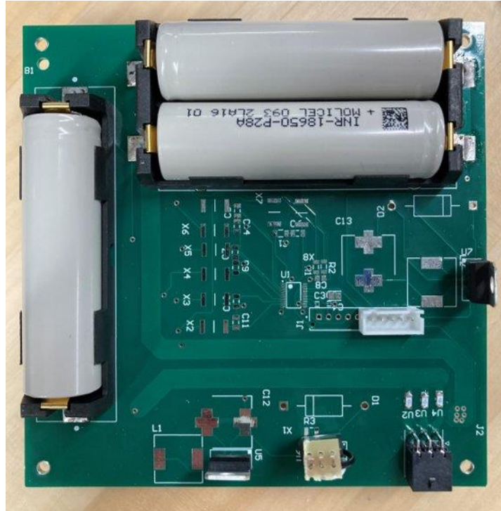
FIGURE 3.40 FINISHED POWER PCB
