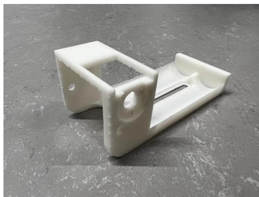
FIGURE 3.15 RIGID RESIN BALL CONTROL MOUNT
