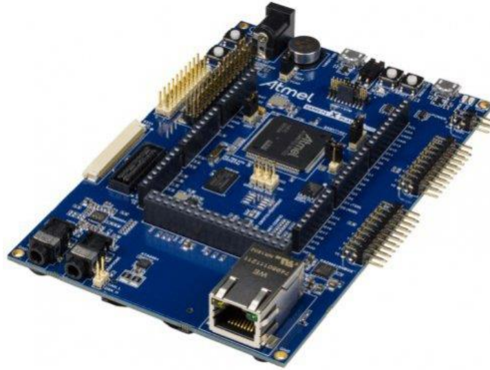
FIGURE 3.21 SAMV71 XPLAINED ULTRA EVALUATION BOARD
