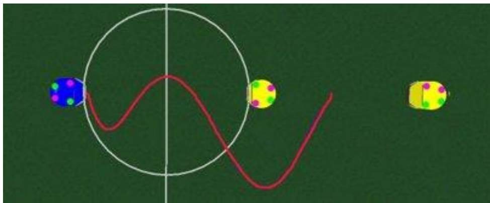
FIGURE 4.16 BLUE ROBOT'S PATH USING RRT* AFTER A POLYNOMIAL CURVE OF BEST FIT IS APPLIED.
