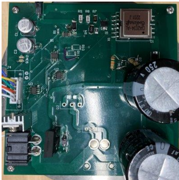
FIGURE 3.39 : FINISHED KICKER PCB
