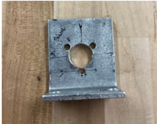
FIGURE 3.35 FIRST PROTOTYPE OF L BRACKETS
