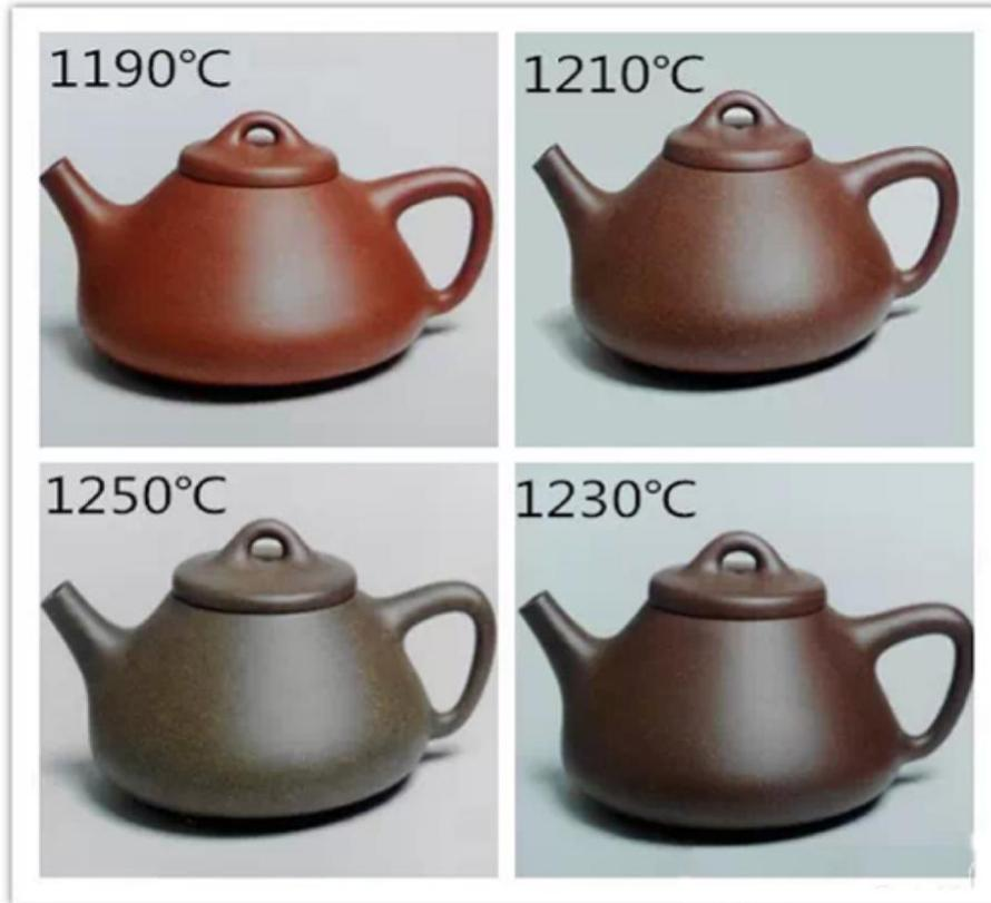
*Figure 6: Different sintering temperature of purple clay (Chao Wang, 2018).*
