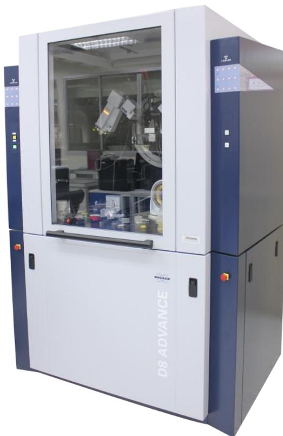
*Figure 15: X-ray diffraction machine (T, 2017).*
