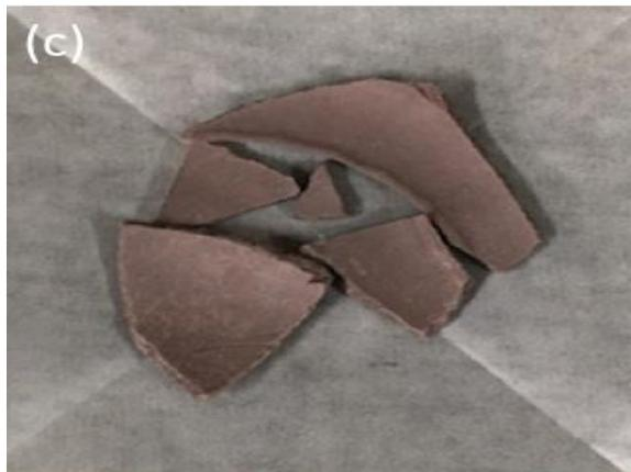
20(c): Non-sintered phase of test sample.
