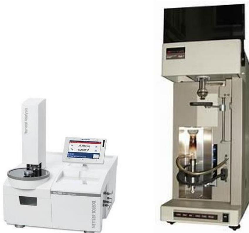
*Figure 16: Thermogravimetric analyzer (U, 2012).*
