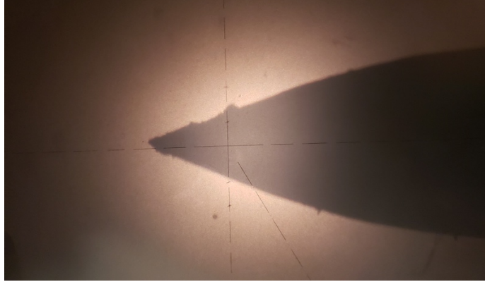
Figure 3.1 - Optical comparator image of convex knife
