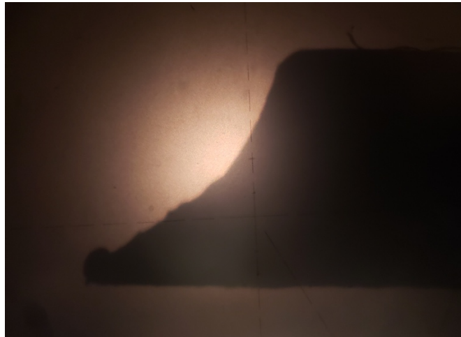
Figure 3.3 - Optical comparator image of curved chip-breaker knife
