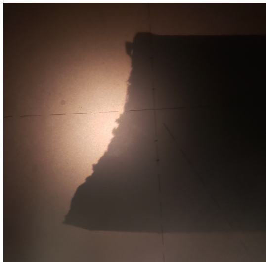
Figure 3.2 - Optical comparator image of (slightly damaged) flat chip-breaker knife
