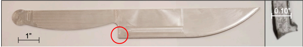
Figure 2.8 - Machined flat chip-breaker blade; Left: front view, and Right: top view of edge feature
