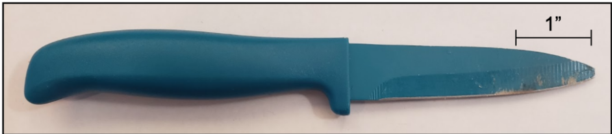
Figure 2.10 - Purchased knife featuring a flat grind
