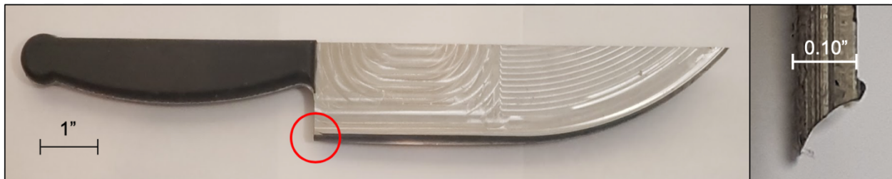
Figure 2.7 - Machined curved chip-breaker blade; Left: front view, and Right: top view of edge feature
