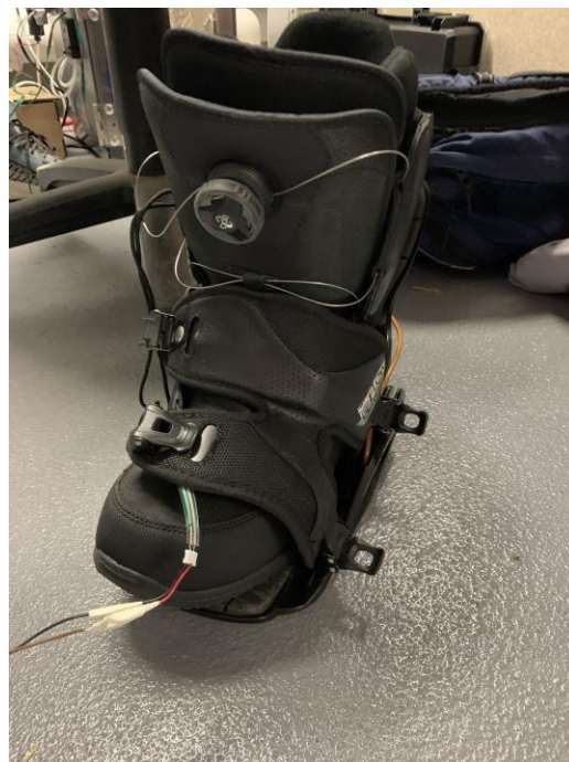
Figure 4.5.3.2 - Rider Detection Sensors Placed Within Appropriate Location within Snowboard Bindings
