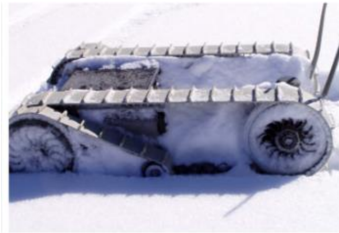
Figure 2.2.3.1 - Buildup of snow in key drive components [9]
