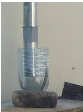
Figure 4.9: Down Pipe and Funnel
