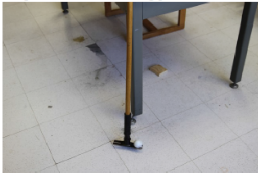
The ball is currently resting on the end of the tool that helps the user set up the golf tee.
