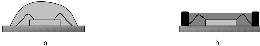
Figure 1.9 Two styles of glob top on ICs (a) single-resin process; (b) two-resin process
