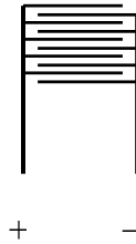
Figure 5.4 An example of a comb structure used to mimic the voltage bias across signal lines during the Resistance to Electrochemical Migration test (IPC-TM-650 2.6.14)
