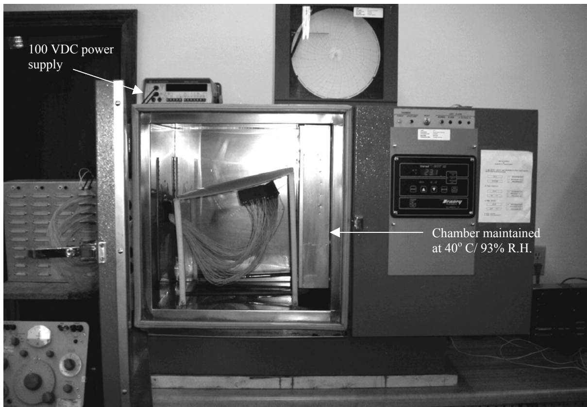
Figure 5.10 Electrochemical migration resistance test set-up, showing test coupons inside of the environmental chamber, connected to a 100 VDC power supply [45]
