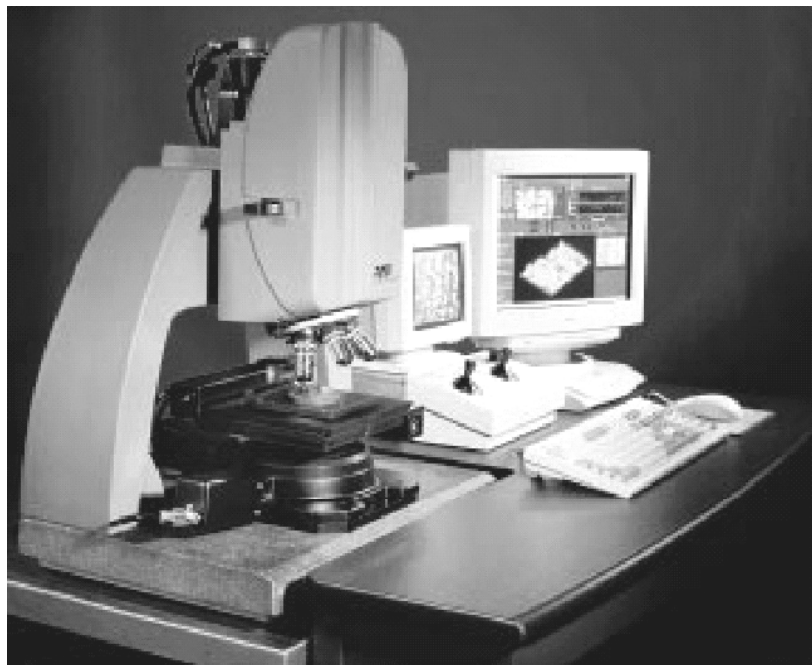
Figure 5.3 Zygo System Advanced Metrology Systems – NewView 5000™ 3D Surface Profiler [43]
