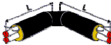
Figure 5.5: Twin Pipe Bend Source: ALSTOM, 2005
