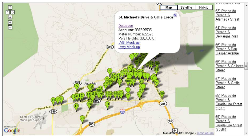
Figure 4: Screenshot of interactive database. Tabs for each signaled intersection provide important lighting information, including PNM account and meter numbers, pole heights and links to CAD and AGi modeling files.
