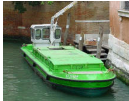
Figure 4.7: Garbage boat with compactor insert
