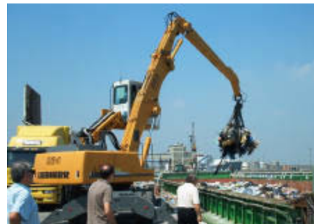
Figure 4.12: Crane with bucket scoop emptying barge into a truck at Fusina
