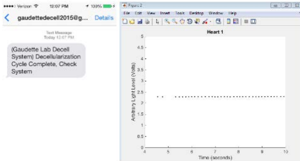
Figure 19: Process Complete Notification and accompanying MATLAB graph of light sensor data.
