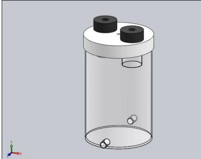
Figure 14: CAD Model of Nalgene Bioreactor
