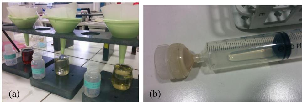
**Figure 8: (a) Filtration with paper filter and (b) filtration with glass microfiber filter**
