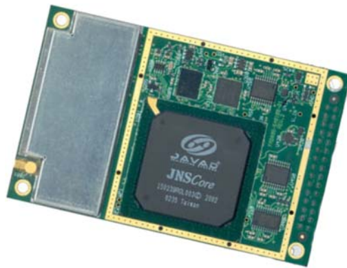
Figure 3.2: WITS GPS OEM Receiver (Source: Javad Navigation Systems JNS100 ) 2
