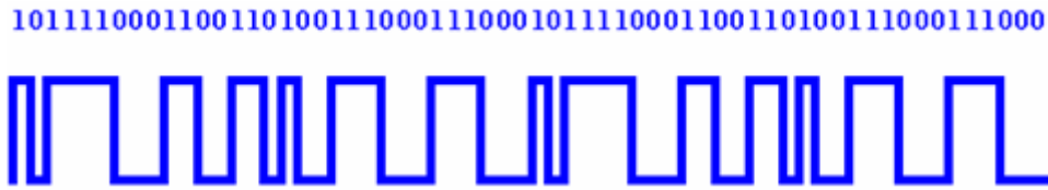
Figure 5.2: Typical PRN_s Sequence Transmitted by a GPS Satellite (Source: Global Positioning Systems ) 4
