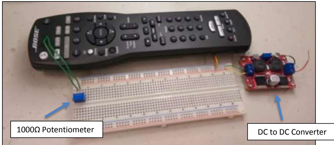
Figure 23: Remote Using Consistent Power Supply and Potentiometer
