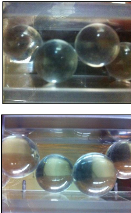
Figure 6: Spiral-Packed Channel Physical Packing. Above: Side View. Below: Top View.
