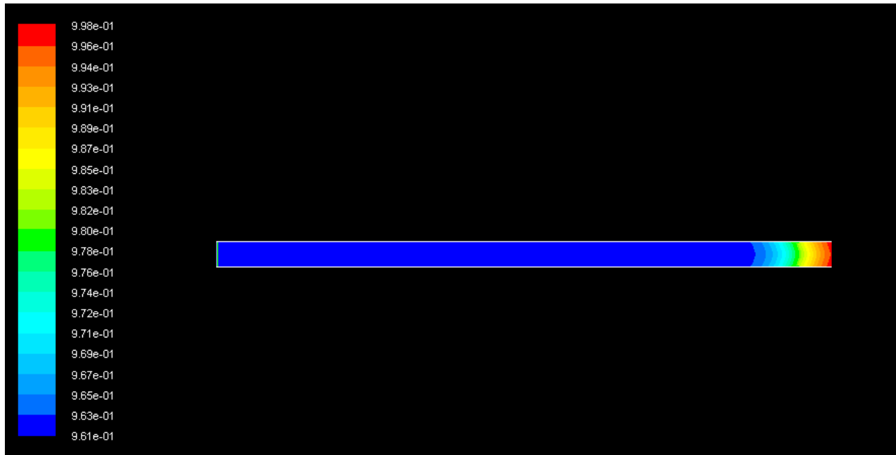
Figure 35: Volume fraction profile of water in 10cm empty channel, 4000 iterations
