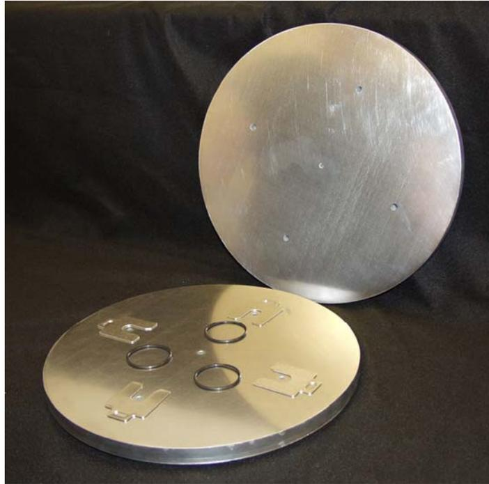
**Figure 11: Compression Set Test Fixture Photograph**
