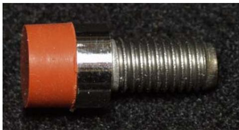
**Figure 20: Photograph of 0.375in. cylindrical adhesion sample attached with cyanoacrylate**
