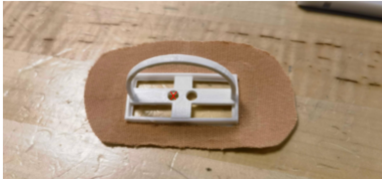
Fig. 13 Base chasing with adhesive applied. The left hole is marked for sampling on the artery.
