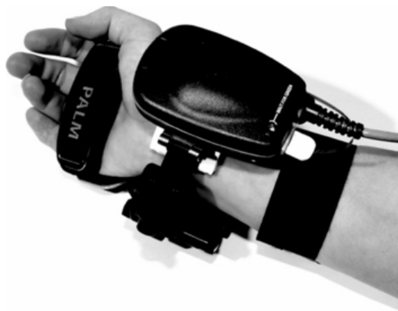
Fig. 4 The T-Line Tensymeter TL100. Automated wrist appliance for measuring BP from the radial artery. [Szmuk et al., 2008]
