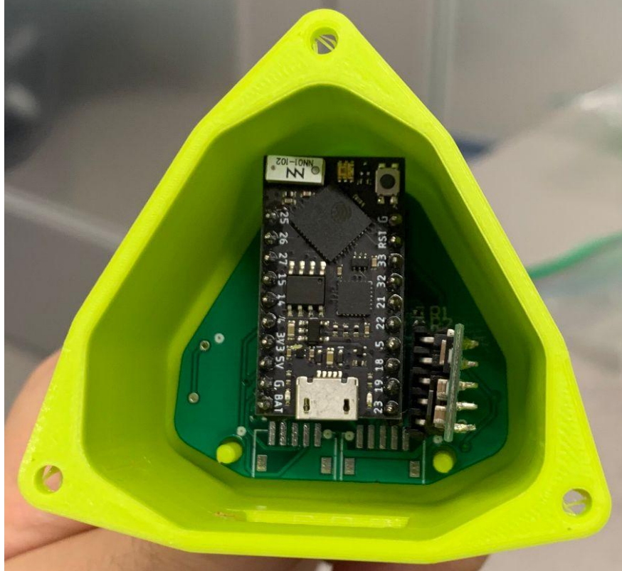
Figure 6: The main board within the new casing without wires; Top View with the 12V step down regulator reoriented
