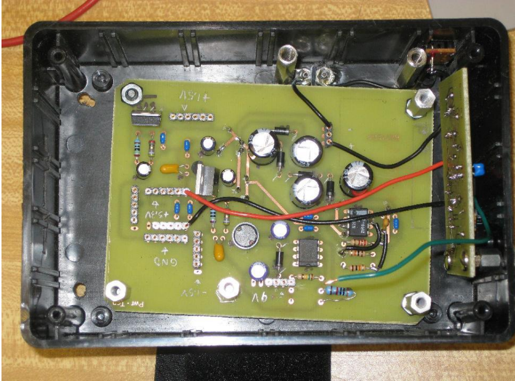
Figure 122: Enclosure - Power and Siren Boards
