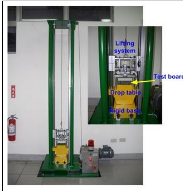
Figure 2-6: Drop Weight Impact Test
