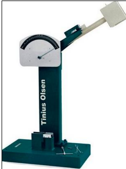
Figure 2-7: Pendulum Impact Test
