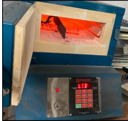
Figure 6.26. 1075 carbon steel sample bar during normalizing cycle.
