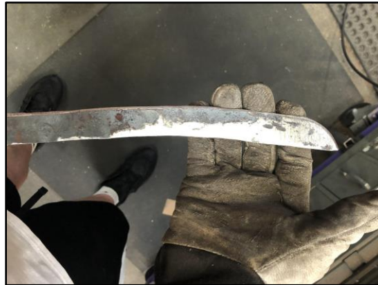
Figure 6.33. Blade after carbon scaling was partially ground off.
