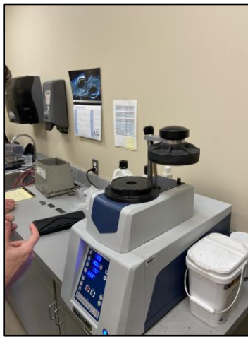
Figure 4.8. Mounting the steel specimens.
