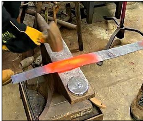
Figure 6.6. The final beveling towards the base of the blade.
