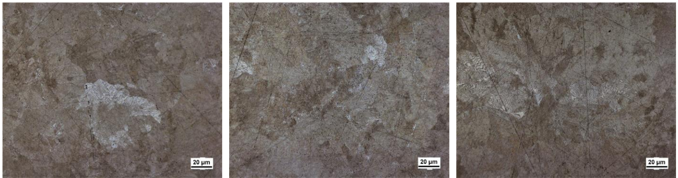
(a) XY plane (b) XZ plane (c) YZ plane Figure 4.22. Microstructure of forged 1075 steel in three planes (500x magnification).
