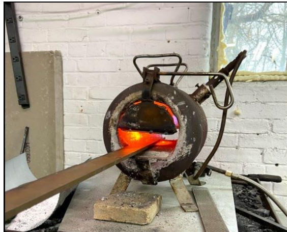
Figure 5.6. Example of a propane forge.
