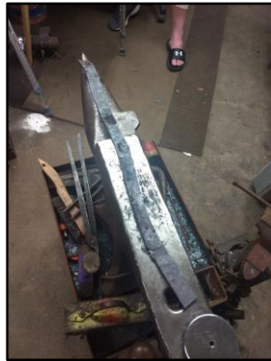
Figure 6.31. Warped blade prior to straightening.
