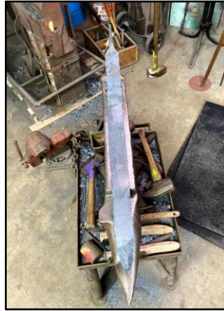
Figure 6.15. The final product after blade was straightened.
