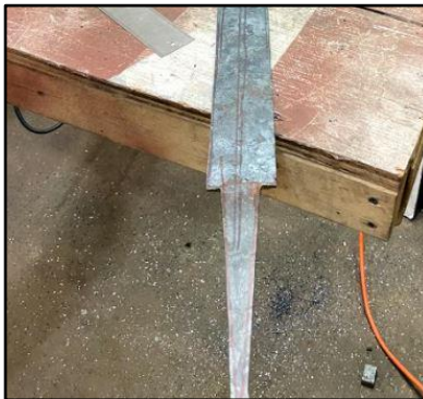
Figure 6.19. The tang after it was fully cut into the blade.
