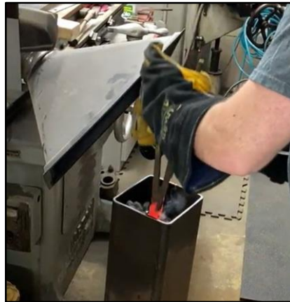
Figure 6.27. Quenching the sample after austenitizing.
