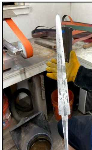
Figure 6.22. The sword bevel almost finished.
