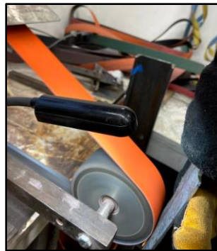
Figure 6.21. Grinding sword bevels with wheel attachment.
