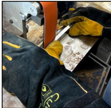
Figure 6.23. Cross guard profile being grinded down.
