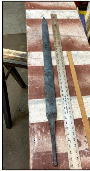
Figure 6.17. The sword after one round of grinding and leveling the edges.
