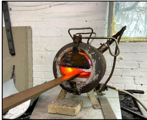
Figure 6.3. Small propane forge heating up.
