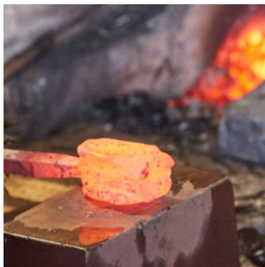
Figure 5.2. Tamahagane welded and folded (JNTO, 2020).
