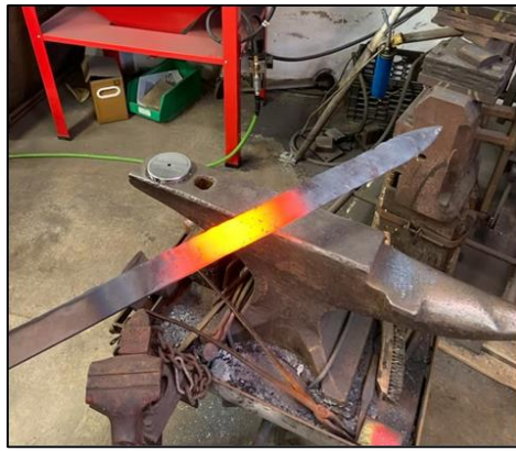
Figure 6.5. Working the bevel down the length of the blade.
