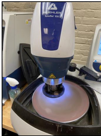
Figure 4.10. Grinding the specimens using different grit sandpaper.
