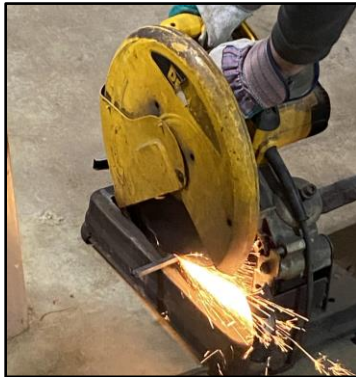
Figure 6.12. The metal cutting saw trimming off metal from the tang.
