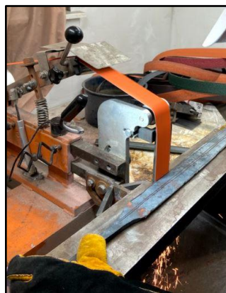
Figure 6.16. The grinding belt setup with the flat table attachment.
