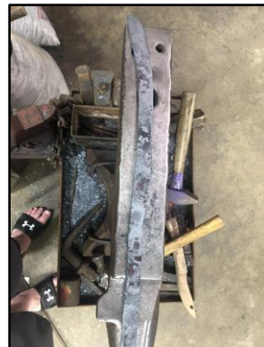
Figure 6.32. Blade after curve was hammered out.
