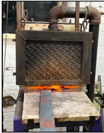
Figure 6.8. The large propane forge with raising doors.
