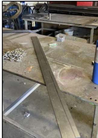
Figure 6.1. 1075 steel marked for plasma cutting.
