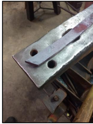
Figure 6.30. Blade with the misshapen tip removed.
