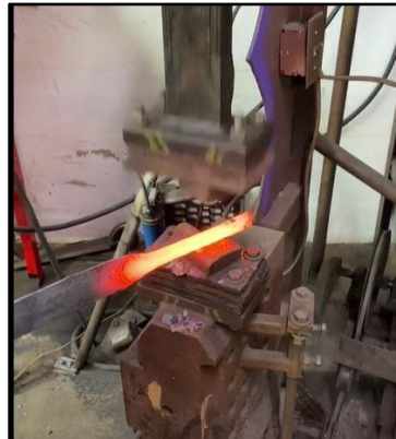
Figure 6.9. The power hammer striking the hot 1075 steel.
