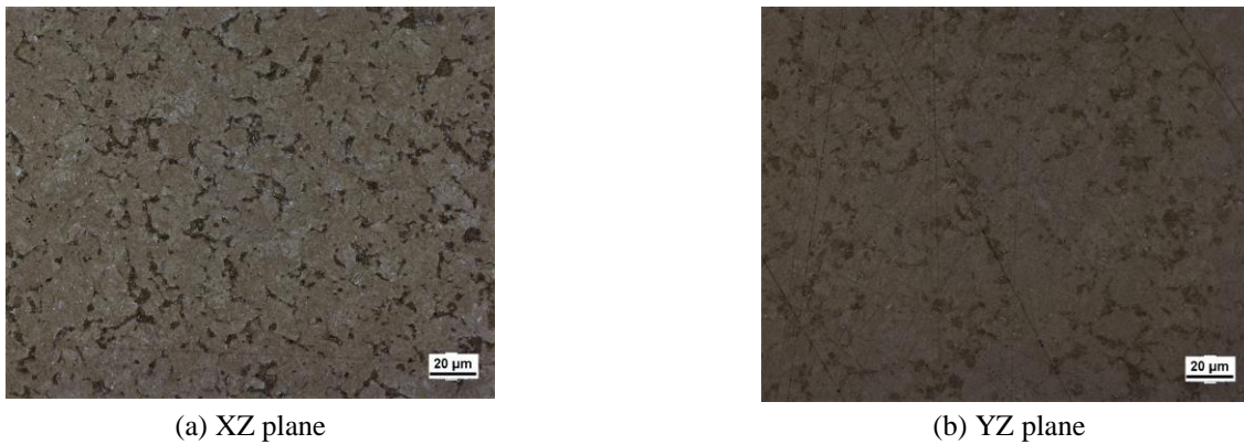
Figure 4.25. Heat treated 1045-1075 combination in two planes (500x magnification).
