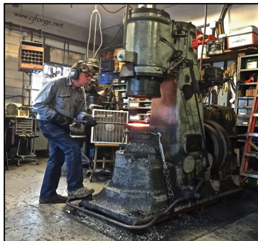
Figure 5.3. Example of an industrial power hammer (Blacksmithing, 2014).
