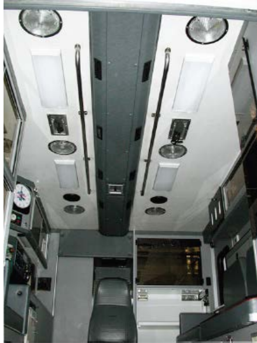
Figure 110 - View of centrally ducted climate control in PL Custom Ambulances
