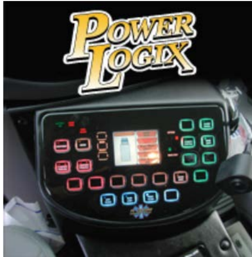
Figure 112 - View of the Power Logix electric system in PL Custom Ambulances
