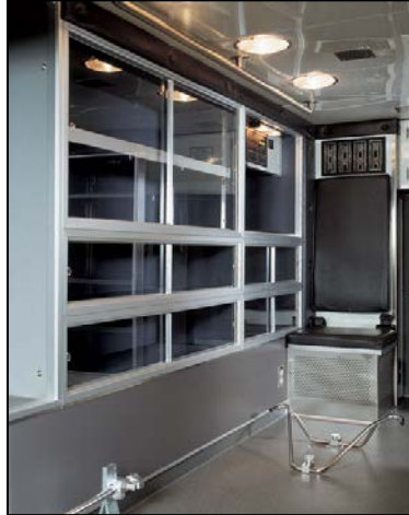
Figure 58 - Type 3 Model 403 Interior Displaying All-Aluminum Modular Cabinetry
