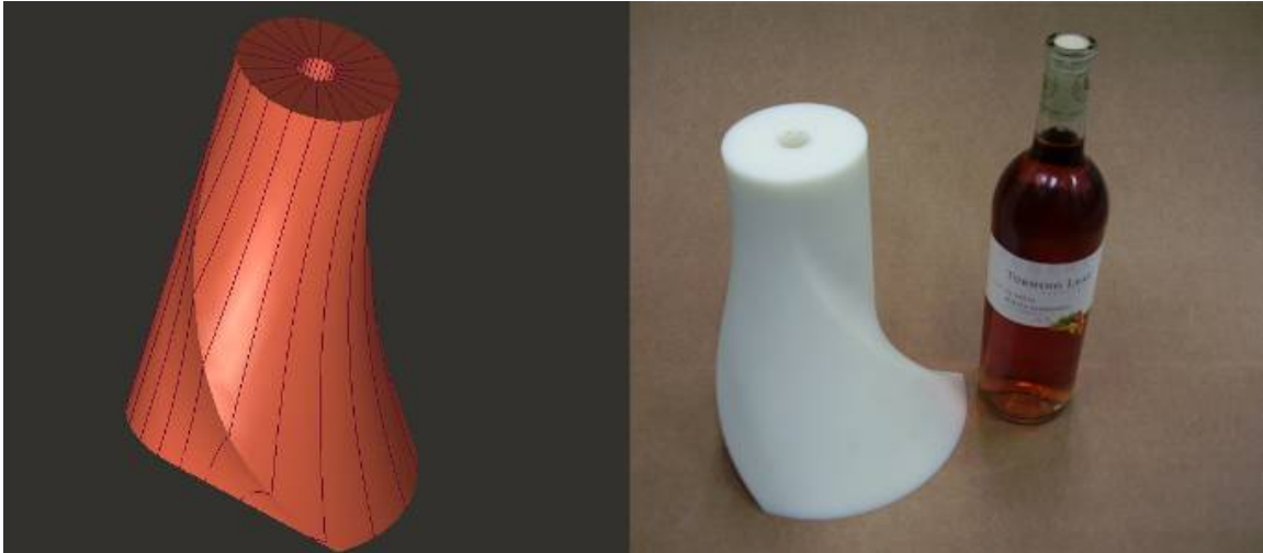
Figure 38: Model vs. Rapid prototype
