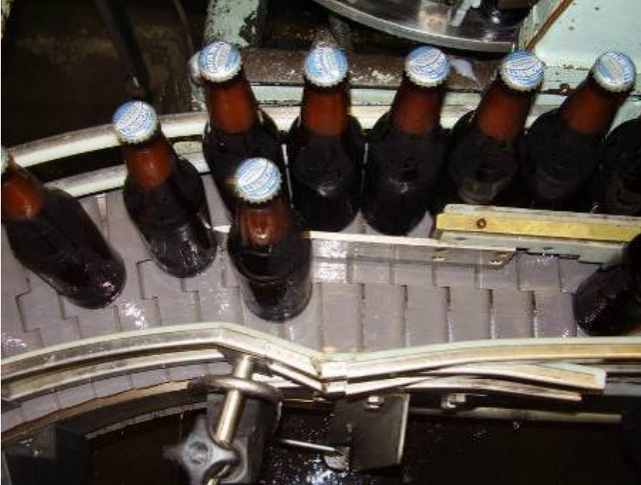
Figure 10: Wachusett Lane Splitter
