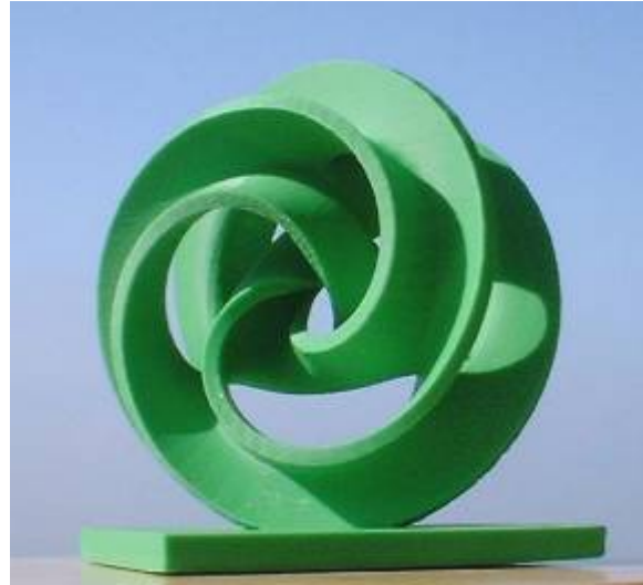
Figure 16: Complex Geometry Realized Through Fused Deposition Modeling
