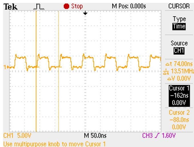
Figure 45 SPI Clock Rate
